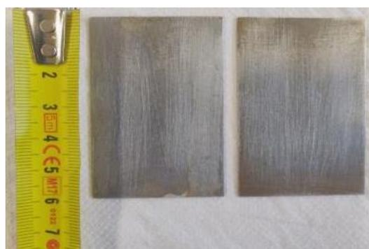
Figure 7 Iron plates used as electrodes for electrocoagulation
