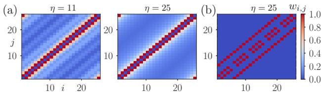
FIG. 3. Engineering of spin models. (a) Long-range interactions  $w_{ij} = 1/|i - j|$  and periodic boundary conditions, for  $\eta = 11, 25$ . (b) 2D nearest-neighbor interactions with open boundary conditions, with  $\eta = 25$ . Here, the indices  $i$  correspond to 2D indices  $\mathbf{i} = (i_x, i_y)$  of a square of  $5 \times 5$  sites using the convention  $i = i_x + 5i_y$ .
