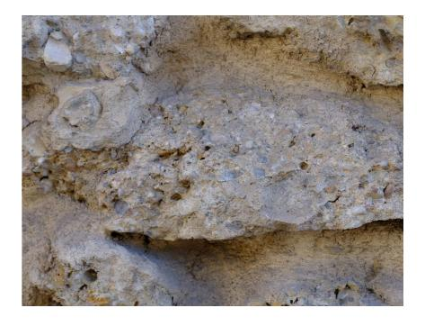
Fig. 3: Weathering of limestone
