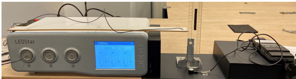
Figure 5.1: The setup for light intensity measurements with the LEDStar on the left, the Konica Minolta illuminance meter on the right and the Konica Minolta illuminance meter receptor head in the middle in front of a ruler with the Eckardt TwinLight placed 20 mm above it by using a small wooden plank.
