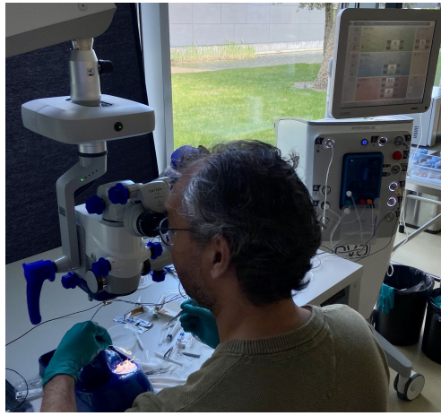
Figure 5.4: Setup for the installation of the RingLight prototypes with vitreoretinal surgeon Koen van Overdam in front of a porcine cadaver eye, about to insert one of the RingLight prototypes. The porcine cadaver eye is placed under a surgical microscope and the RingLight prototype is connected to the EVA eye surgical system on the right (also used for vitrectomies).
