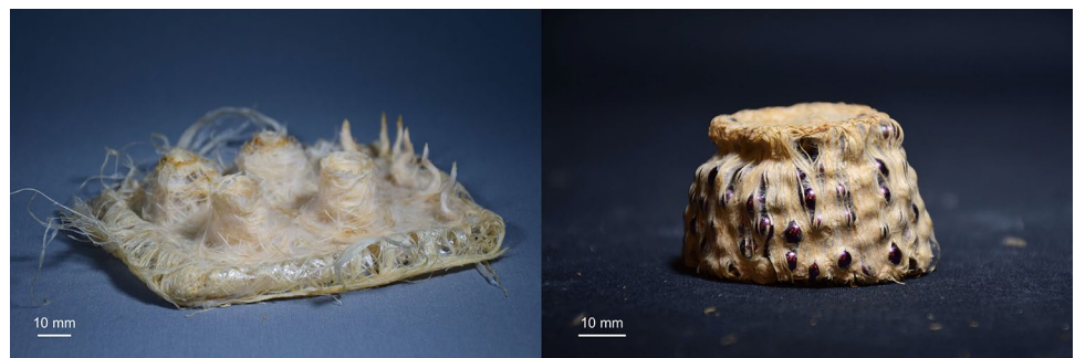
Fig. 9 3D forms grown by roots (left); 3D form co-created by roots and 3D barriers (right)
