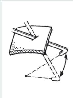
A rigid 90° endoscope can be used to view organs from several sides. One drawback is that the image will be tilted, resulting in a slight orientation error. This calls for another solution, i.e. a steerable tip.
