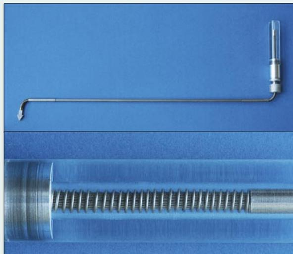
Overall view of the third prototype of the Endo-Periscope.
