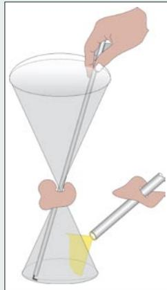
The incision acts as a fulcrum for the movements of endoscopes and instruments. As a result, movements of the hand are both mirrored and scaled.
