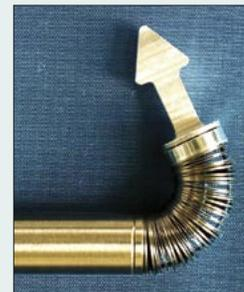
Breedveld's second prototype of the Endo-Periscope, developed in 2001-2002 had a diameter of 12 millimetres. The significant features of this model are the simplified construction of the grip and the parallelogram mechanism.
