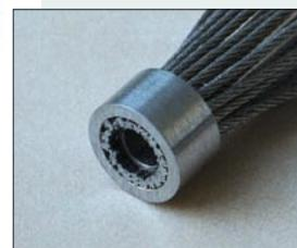
Close-up of a model to test the fixation of the 22 cables between the two rings.
