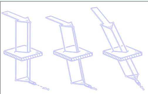
The principle of the Endo-Periscope is based on parallelograms. The camera (at the bottom) accurately follows every movement of the grip.
