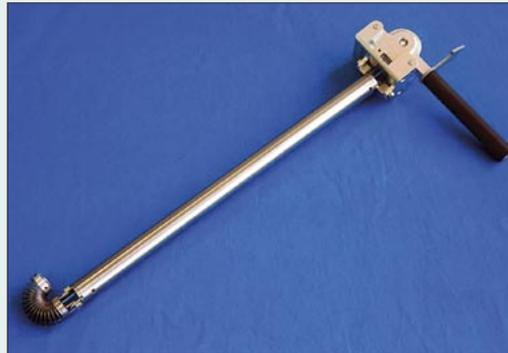
The endoscope tip can be rotated sideways from  $-60^\circ$  to  $+60^\circ$  (left), and up and down between  $0$  and  $180^\circ$  (right).
