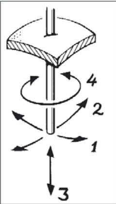
The cut in the abdominal wall restricts the motion of current rigid endoscopes to one translational and three rotational degrees of freedom.
