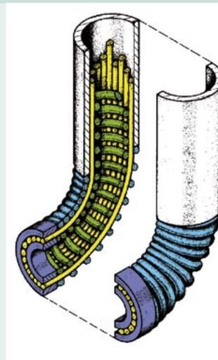
Cross-section of the tip of the recently developed third prototype of the Endo-Periscope, showing the ring of cables, surrounded by two helical springs and fixed at the tip between two rings.
