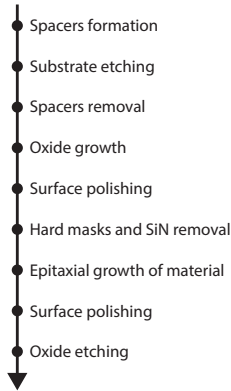
Figure 2.12: Replacement fin patterning process flow of FinFETs on bulk wafer.
