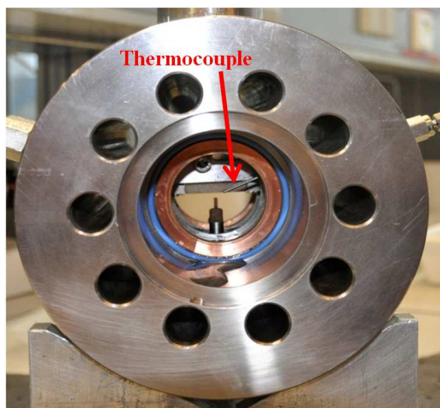
Figure 2.3. Side view of the open pendant-drop cell showing the location of the gas inlet tip and the thermocouple inside the cell
