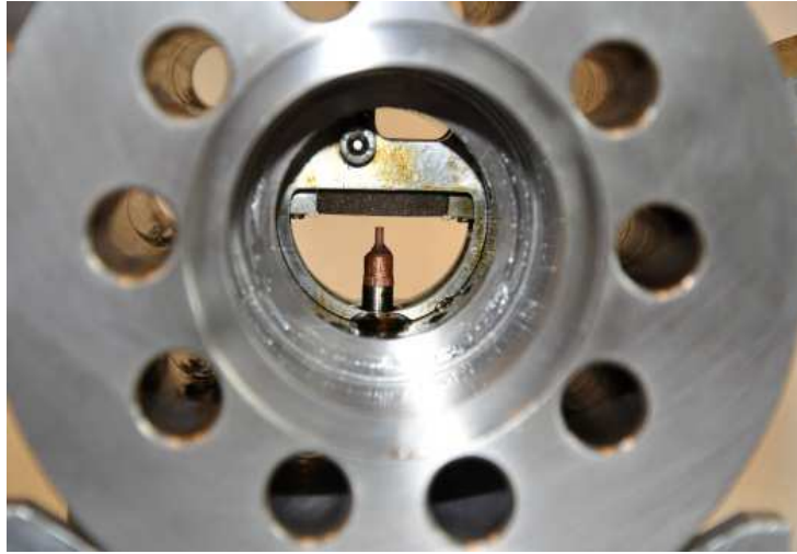
Figure 5.1. Digital photograph of the inside of the modified pendant-drop cell with a Bentheimer Sandstone sample mounted inside. At the bottom the injection tip with an outer diameter of 1.8 mm is observed.
