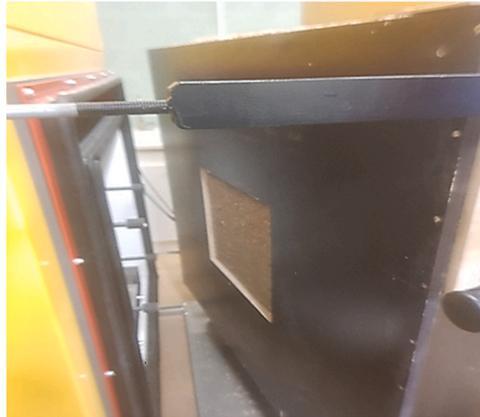
Fig. 12. S/BP wall insertion in the Thermo<sup>3</sup> device.
