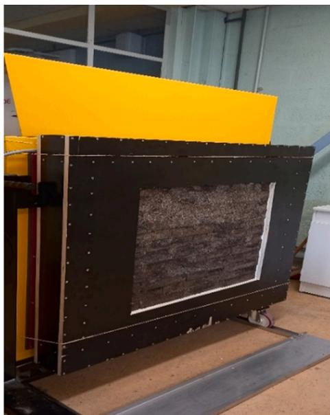
**Fig. 15.** S/BP wall fixed from one side to the hot climatic chamber and exposed to ambient temperature from the other side.
