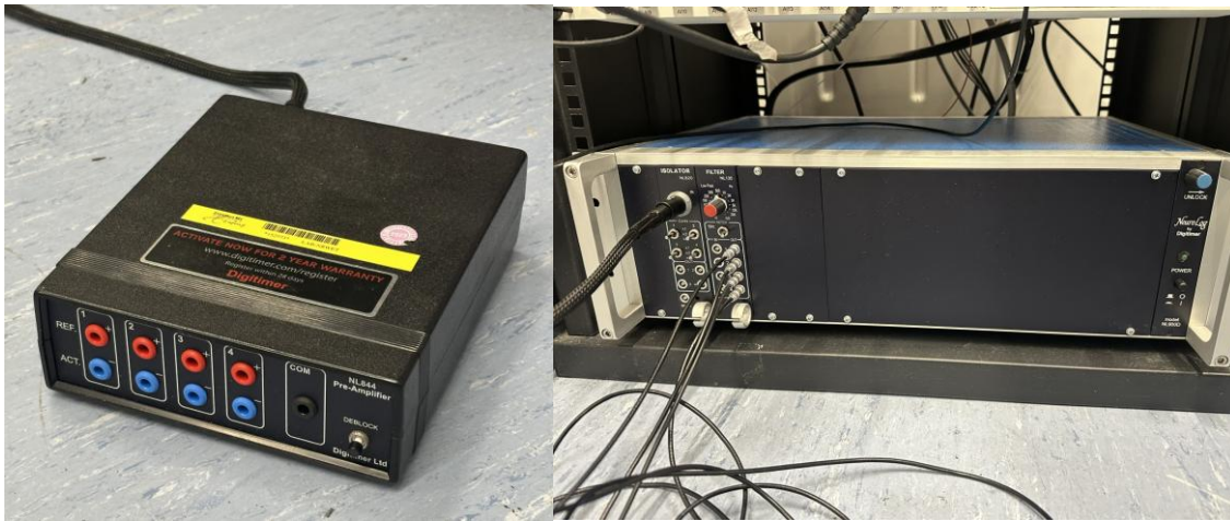
Figure 14: pre-amplifier (NL844, Digitimer) (left) and filter and isolator (NL135 filter, NL820 isolator, Digitimer) (right) with which EMG measurements were taken.
