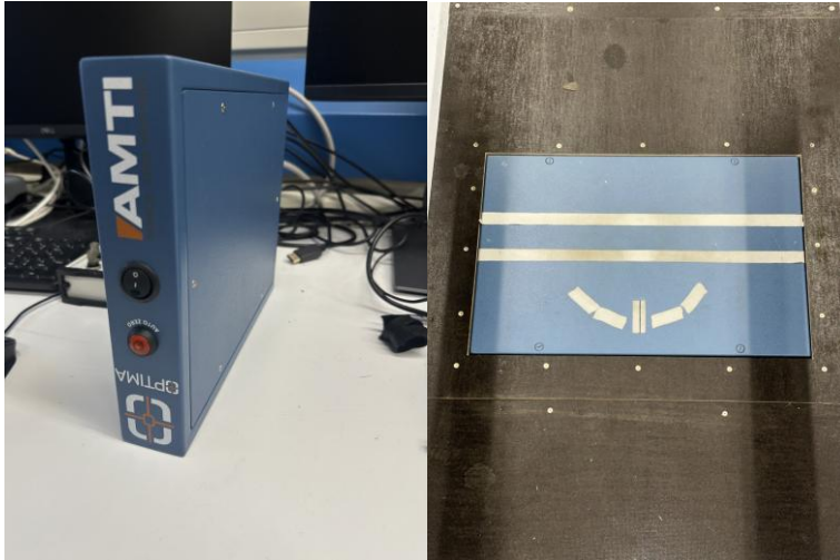
Figure 13: Force plate amplifier (Optima OPT-SC, AMTI, MA, US) (left) and force plate (BMS 400600HF-1K, AMTI, MA, US) (right). The horizontal tape was used to outline the participants in anteroposterior direction.
