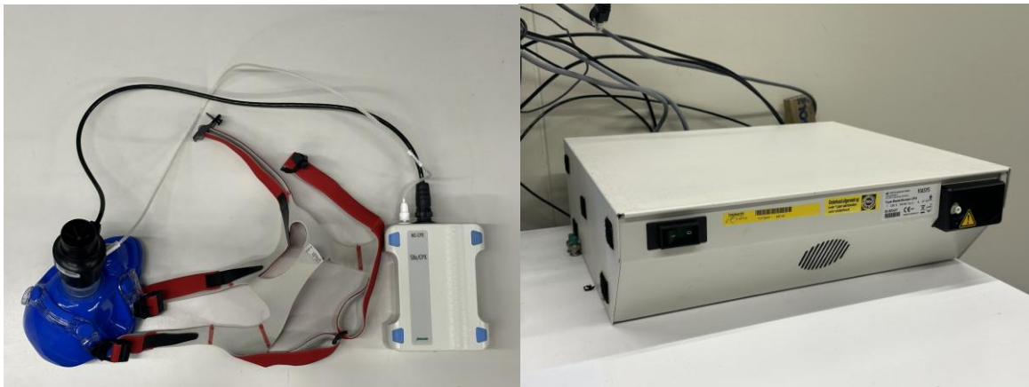
Figure 11: metabolic mask (V-982185, Vyair Medical, USA) where flow and gas measurements are captured and which is connected to the wearable metabolic device (SBx/CPX, CareFusion, USA) (left). The wearable metabolic device was connected to the indirect calorimetry system (MS-CPX, VIASYS, Germany) (right).
