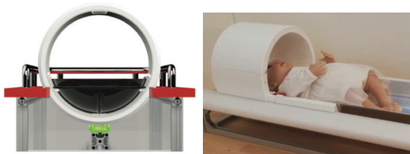
Fig. 11. The suspended coil in front view. The black part is the headrest, the red part is the top plate of the bed, green is the sliding rails. The coil is only suspended on the top plate and not attached to the rails (left). Patient positioning (right) [8].
