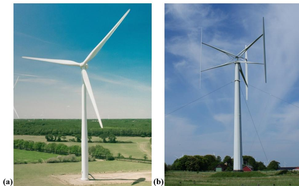
**Figure 2.1:** Two types of wind turbines, (a) a horizontal axis wind turbine (HAWT) and (b) a vertical axis wind turbine (VAWT), specifically an H-rotor. Images from [34] and [35].
