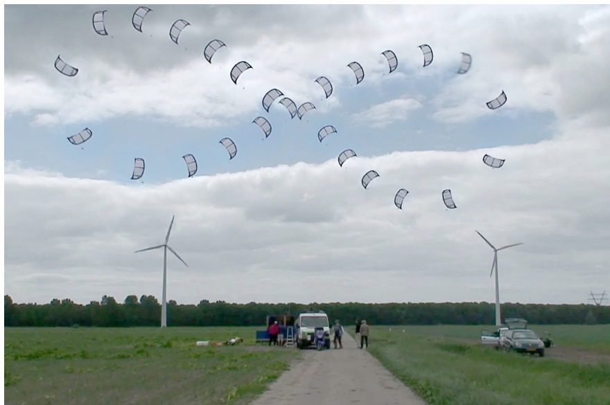
Figure 2. Composite photo of a crosswind figure-of-eight maneuver ( \Delta t = 1 s) of a tube kite with 25 m 2 wing surface area [9].
