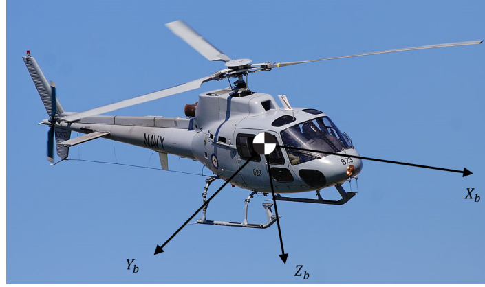
Figure 2-10: Definition of Body-fixed reference frame F_b [3]
