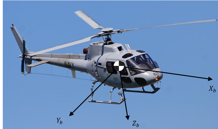
Figure 2-4: Definition of Body-fixed reference frame F_b [3]
