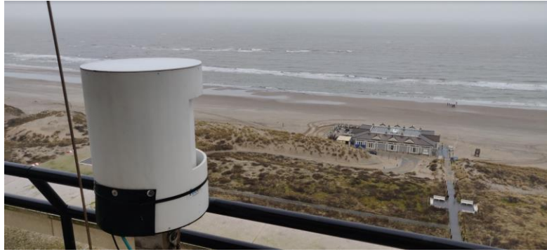
Figure 3.2. The Riegl VZ-2000 on top of the balcony of Grand Hotel Huis ter Duin with its corresponding view over the beach
