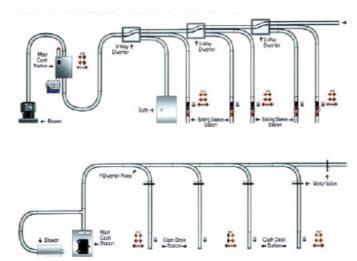
Figure 39: Two-way pneumatic tube system; point to multiple points and vice versa 65
