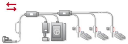
Figure 38: Two-way pneumatic tube system
