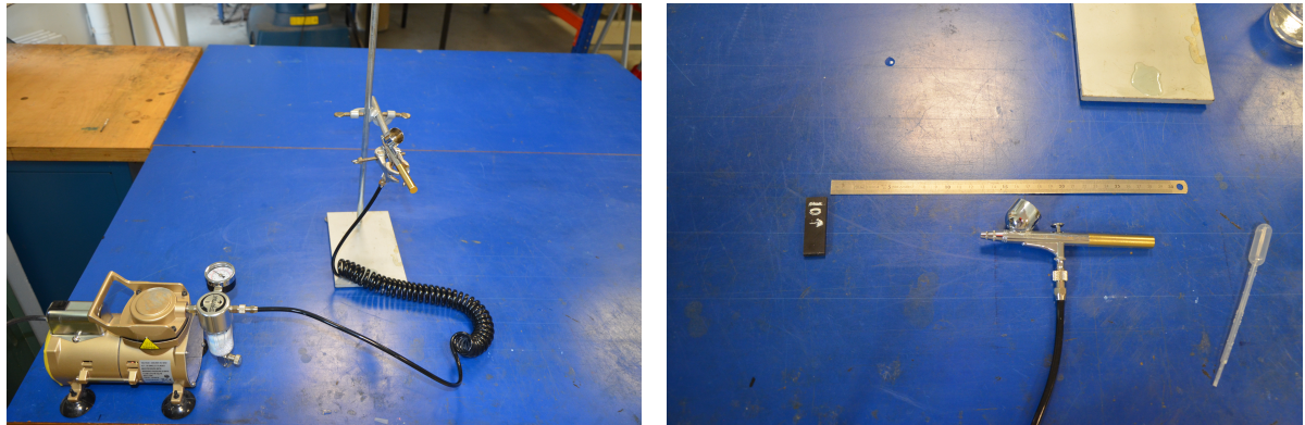
(a) The overall components of the airbrushing system: compressor, connector hose and spray-gun. (b) Close-up of the spray gun and a specimen.
