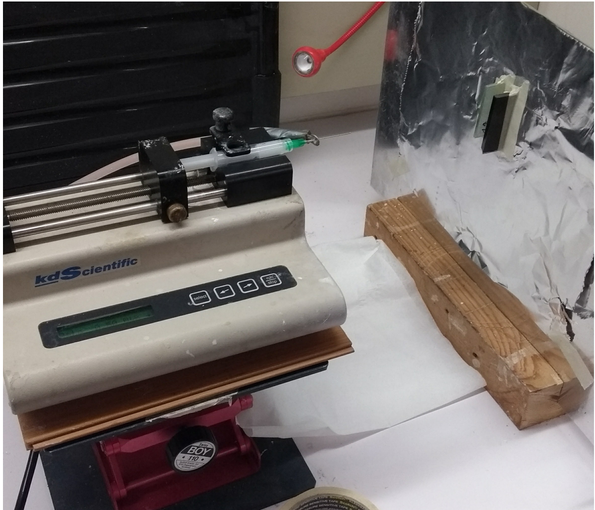
Figure 3.5: The electrospraying setup.
