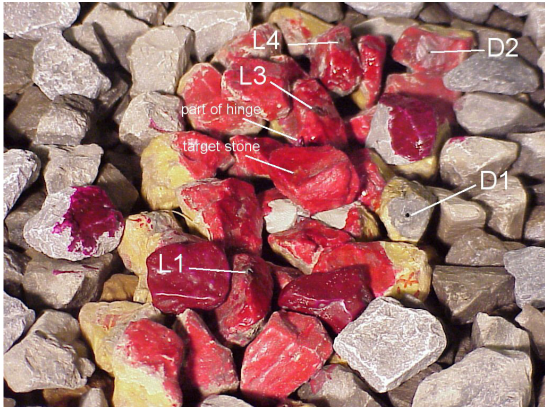
FIGURE 3.6 Close-up of the artificial stones and the visible parts of the built-in measuring devices.
