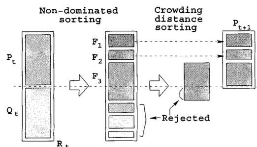
Figure 7.3: NSGA-II procedure
