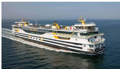
Figure 8.2: Double-ended road ferry TESO Texelstroom with two bridges. Source: figure obtained from [13].
