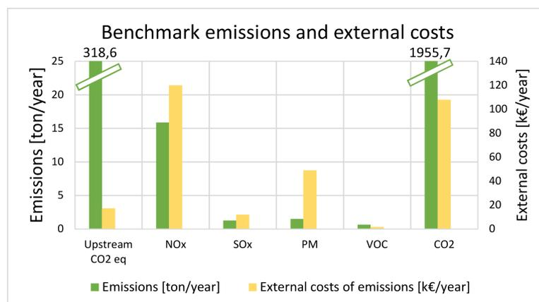
Figure 9.3: Benchmark (workboat) emissions and external costs, with the external costs shown on the secondary axis
