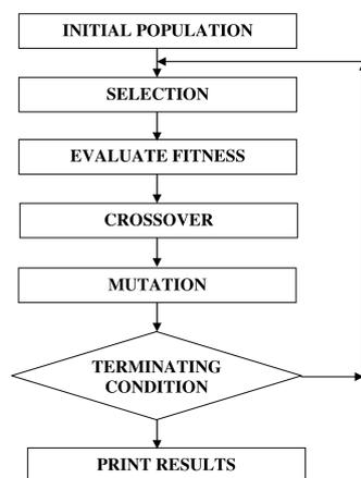
Figure 7.1: Loop of a genetic algorithm
