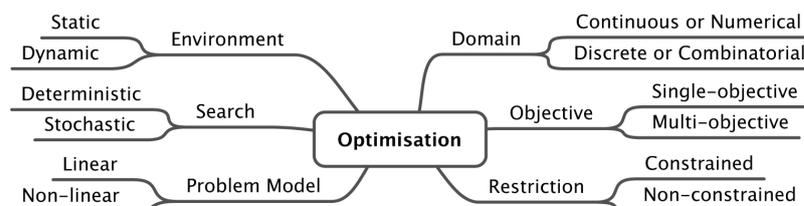
Figure 4.2: Aspects of an optimisation problem. Source: figure obtained from [37]
