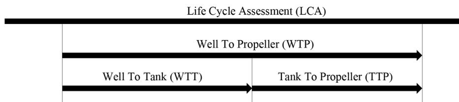
Figure 2.1: Considered emission stage (WTT and TTP)
