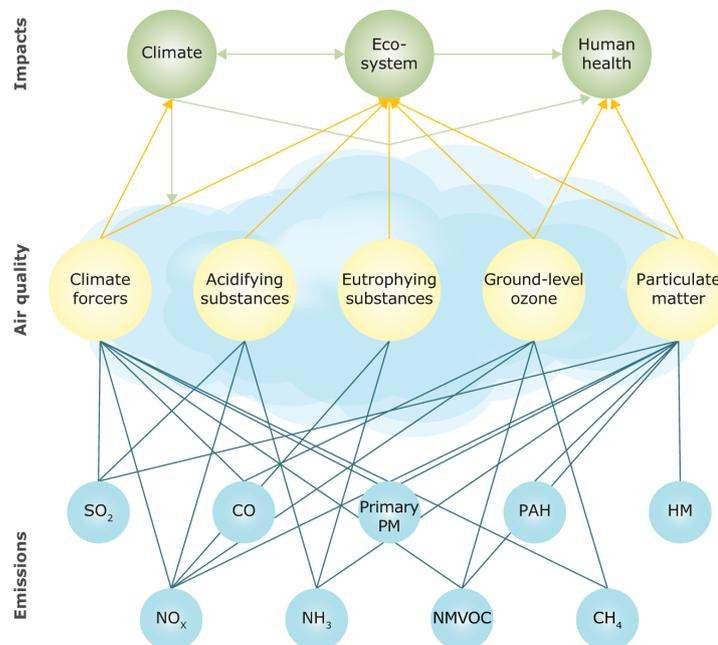
Figure 2.2: Various effects of air pollutants clustered according to impacts (Climate forcer: pollutants that interfere with Earth's energy balance [31]). Source: figure obtained from [31]
