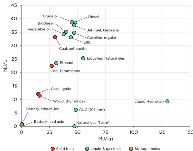
Figure C.1: Volumetric and gravimetric density of fuels and storage media. [40]
