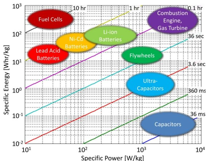
Figure B.1: Ragone plot of energy systems, the axes are logarithmic. Source: figure obtained from [32]
