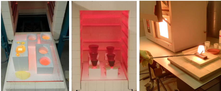
a) Kiln-casting in Crystalcast moulds with glass directly placed in the moulds (free-set), b) Kiln-casting in Crystalcast moulds employing the flowerpot technique, and c) Hot pouring in steel mould.
