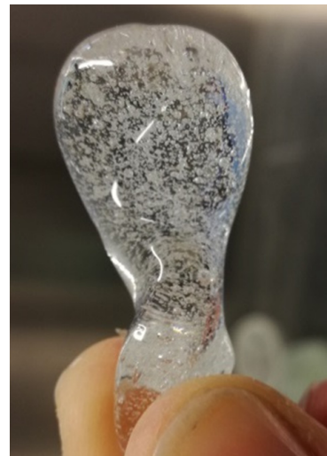
d) Melted at 1500°C in a high-alumina crucible and poured into a steel mould
