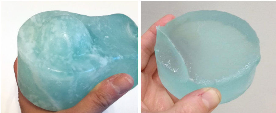
Aquamarine glass cast at 860°C and 1200°C respectively
