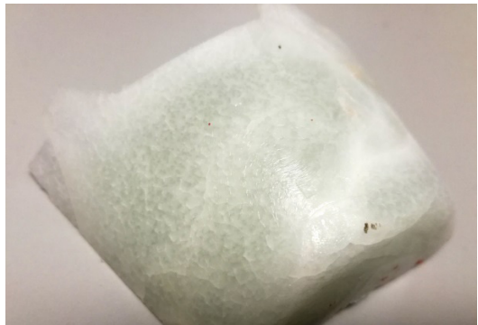
b) Glass part that fused inside the flowerpot. In this picture, the surface in contact with the flowerpot is seen
