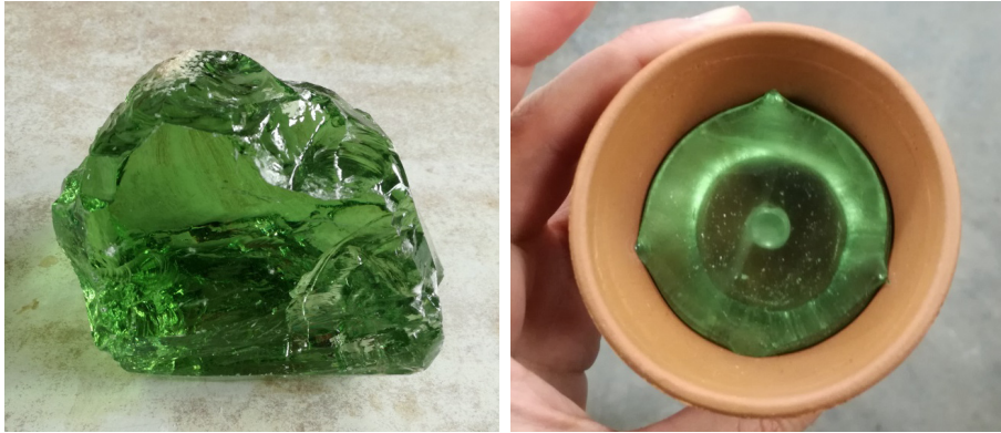
Green glass before and after casting at 860°C
