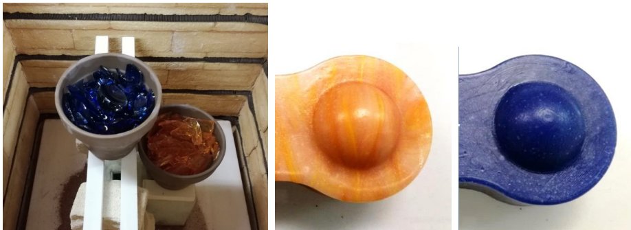
Figure 10: Set-up of the kiln and glass ceramic samples resulting from the mouth-blown glass waste
