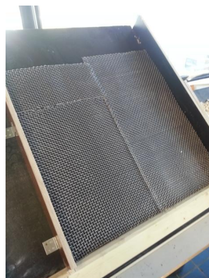
Figure 3-11: Iron mesh for dry pull test
