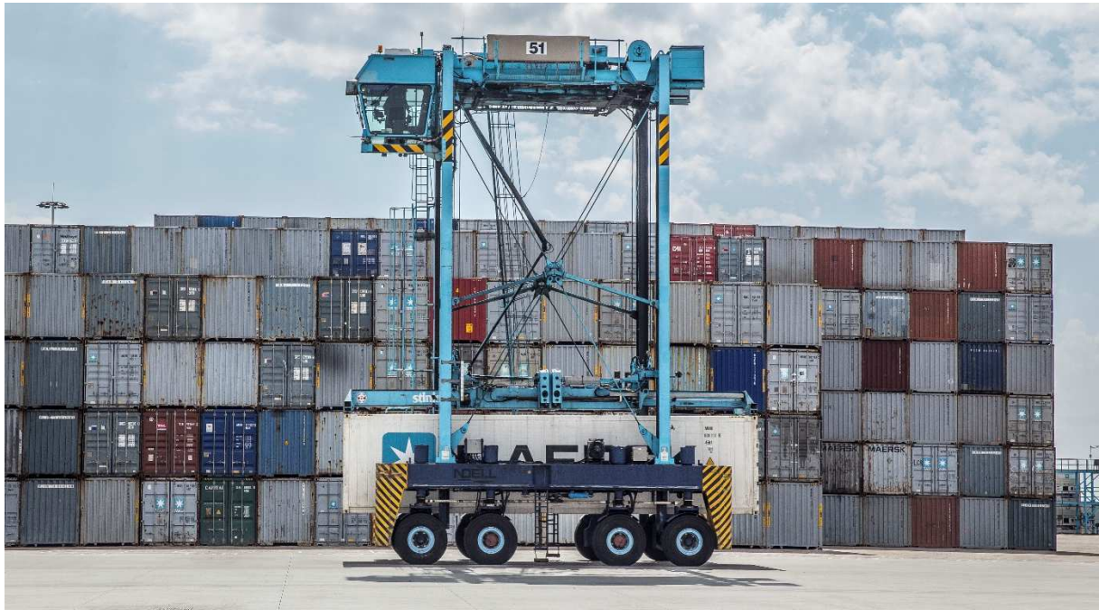
Figure 10 - A Noell straddle carrier (source: APMTR)
