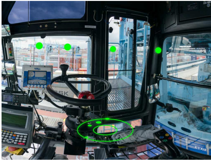
Figure 36 - Concept 1: Augmented reality - left: drivers view, right: head mounted display (source: Vuzix)
