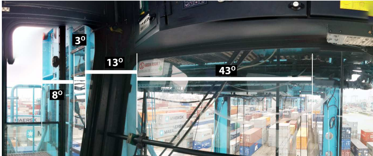
Figure 57 – Angular size estimates port-side blind spot seen from driver position
