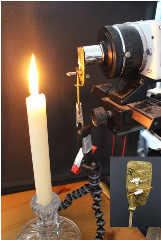
Fig. 8 Setup used for photography and filming with the facsimile microscopes and an eyepiece adaptor in place of the macro lens used in other experiments. From left to right: candle as light source, facsimile van Leeuwenhoek microscope in clamp, Canon EOS M10 camera body fitted with eyepiece adaptor. Inset: the back of the microscope with copper wire attached to aid fine focus. Robertson (2019)
