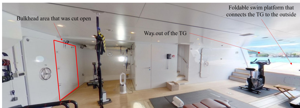
Figure 8.3: Sport's TG showing the bulkheads AO and the way out (adapted from Edmiston, 2024)
