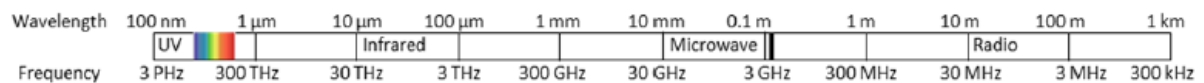
Figure 2.1: The electromagnetic spectrum showing both frequency (Hz) and wavelength (m). The visible light is indicated by the rainbow colored pattern and the black bar indicates the operating frequency of Bluetooth systems. Source: Mautz [23].
