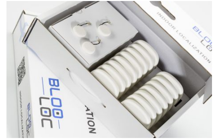
Figure 2.7: The BlooLoc Starter Kit, 1 basestation, 15 beacons and 3 tags. Source: BlooLoc [2]
