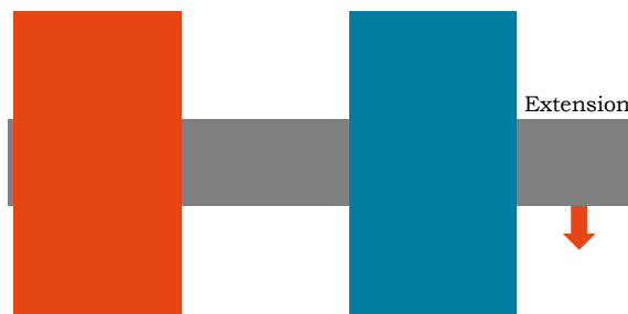
Figure 6.3: Design adjustment shown; heat pipe with condenser side of heat pipe extended. Cold strip is shown in blue and hot strip in red. The red arrow indicates heat loss from the extension.
