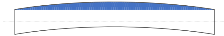
Figure 3.13: Eccentricity with axis of rotation(dashed) and filling compensation for eccentricity(blue). The eccentricity has been drawn in an enlarged way.
