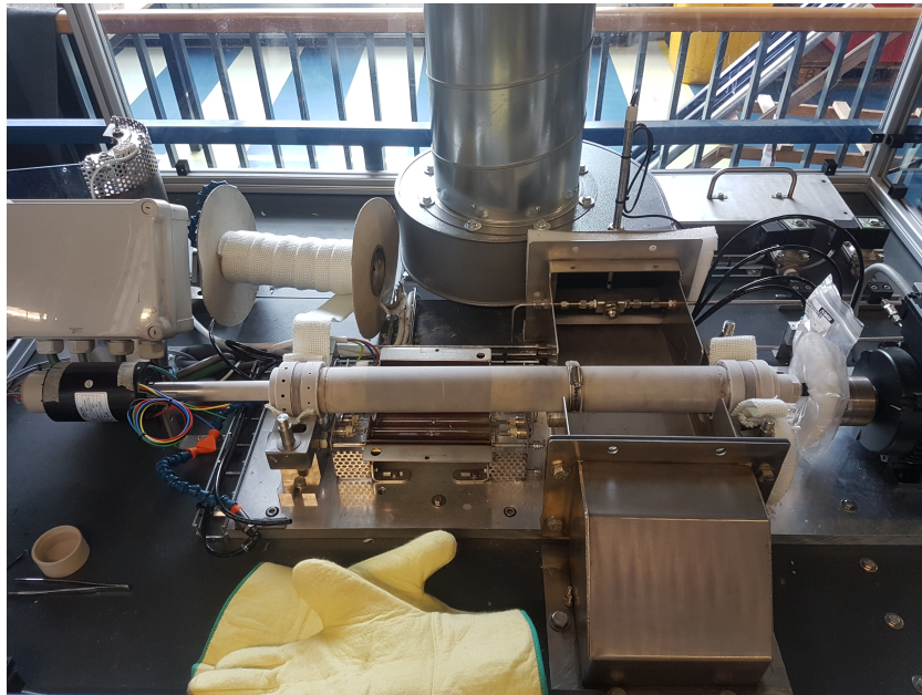
Figure B.1: Heat pipe just out of climate chamber/freezer, with insulation at contact areas and slip ring connected
