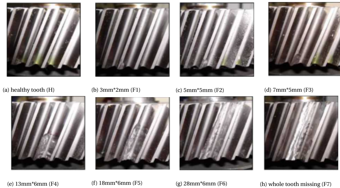
Figure 3.6: Gear tooth damages induced in the gearbox pinion of the WTCMTR [19].
