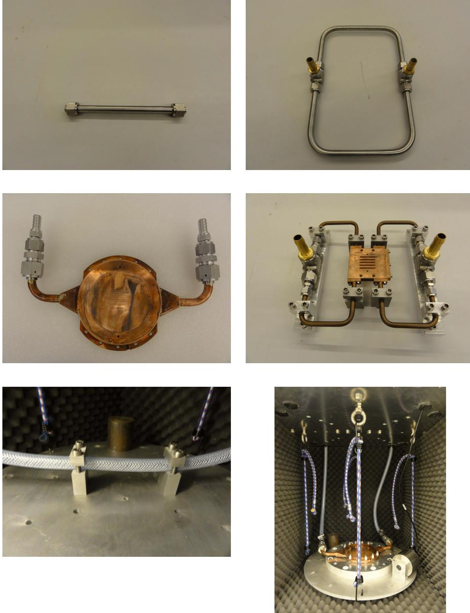
*Figure C.2: The components characterized on Vibronix: The straight tube (upper left), Rectangular component (upper right), Aperture Array (middle left), Dummy Aperture Array (middle right) and tubing connected to plate (bottom left). In the bottom right the AA is shown mounted in Vibronix.*
