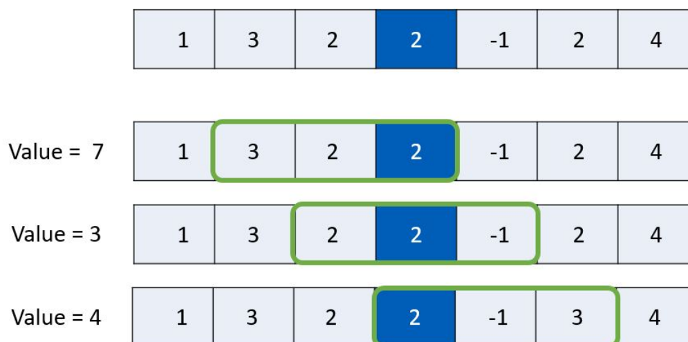
Figure 1.16. Illustration of the Maximum Neighbourhood Value Method. Initial block in dark blue. Green rectangles indicate possible neighbourhoods with their value indicated on the left. Based on Ataee-pour (2005)
