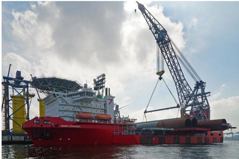
(a) Typical Installation Vessel - Seaway Strashnov
