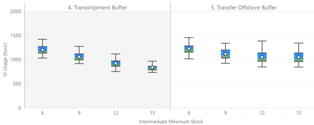
Figure 6.19: Installation vessel usage duration with different minimum stock levels
