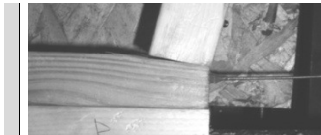
figure 60: Compression perpendicular to the grain at ultimate load in a shear-wall test. (NAHB Research Center, 2003)
