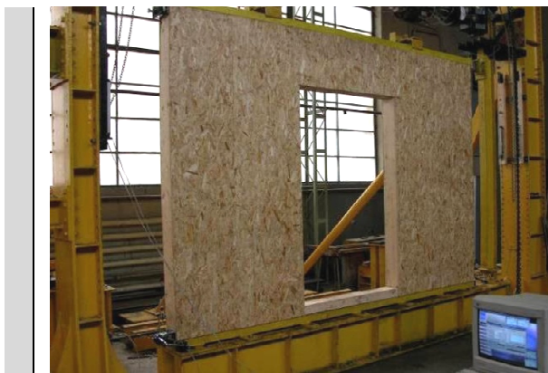
figure 87: Illustrative test-setup to determine the load-displacement characteristics of a perforated timber-frame shear-wall. (Fülöp et al., 2006)
