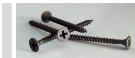
figure 30: Standard drywall screws \varnothing 3,8 \times 45 . d_{ef} = 0,66 \cdot 3,8 = 2,51 mm
