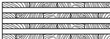
Figure 5: Cross laminating timber layers (cross sectional view) (Znabei, T., 2020)
