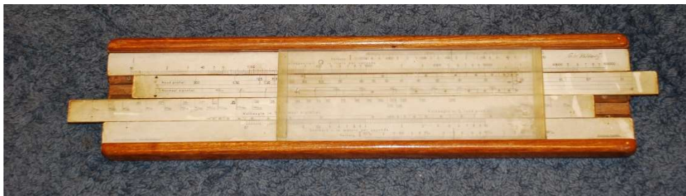
Figure 1.5 Sewerage rule (Riolschuif), developed by K. Kaspers (Note: H. van Mameren, personal communication, 23 September 2021. Copyright 2021 by H. van Mameren. Reprinted with permission).
