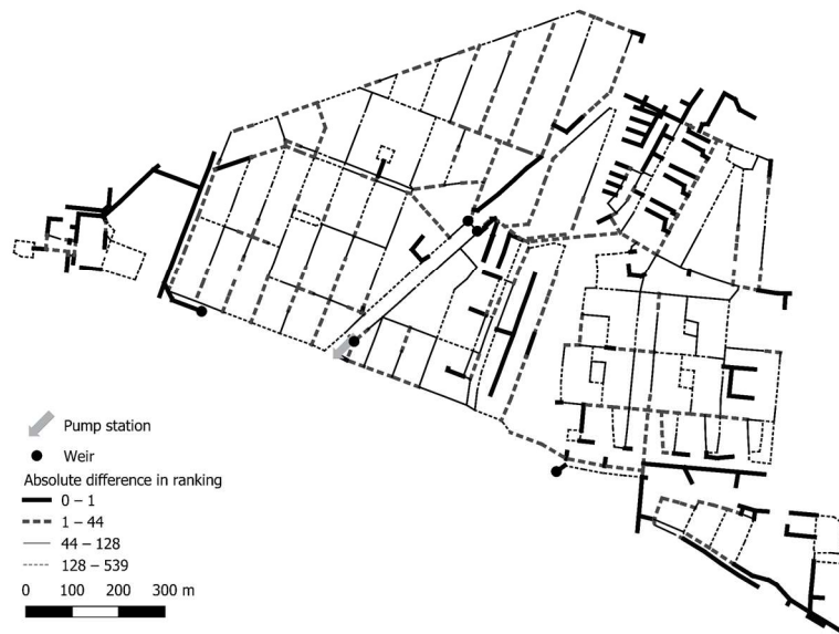
Figure 6.13 Difference in criticality rank between the hydrodynamic model-based weakest link method and the graph theory method for Tuindorp. The classification of the groups is based on the equal count method.
