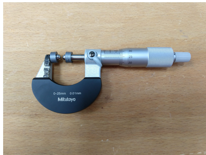
Figure A.9: Two bearings are connected to the micrometer to ensure that the thickness of the shell is measured with a point contact
