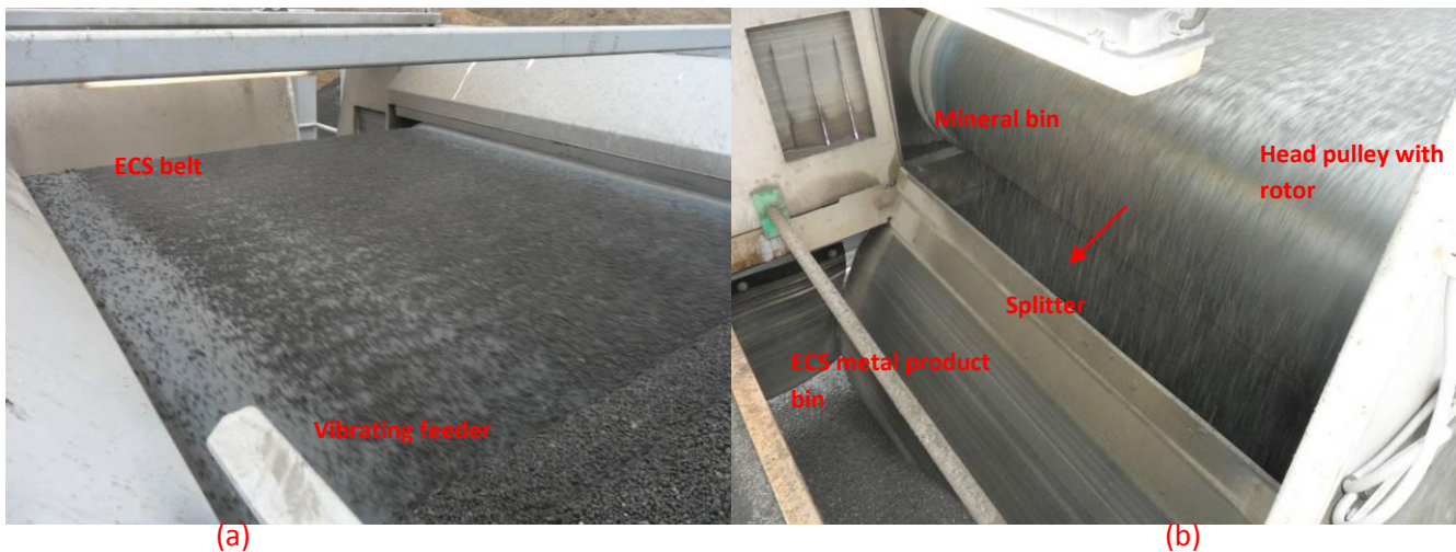
Figure 9: (a): Left an example of an ECS for the 1-6 mm fraction with the vibrating feeder. (b) The right picture shows the product discharge area. Source: Inashco, 2013.
