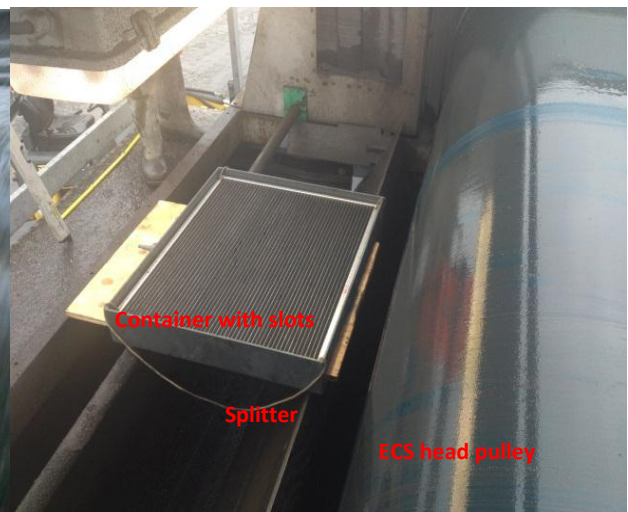
Figure 23: (a) Experimental trajectory measurement in-situ. (b) ECS falling product stream. (c) Experimental setup
