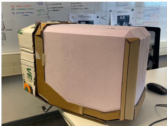
Figure 8.16, 8.17 & 8.18 | Cardboard on foam prototyping.
