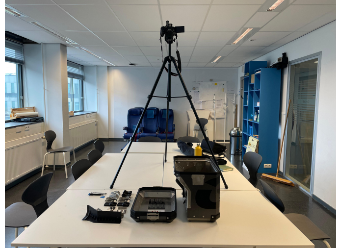
Figure K1 | Setup of the gentle dismantle - Video camera to record the process, tools, and the LSS of the BMW R 1200 GSA.
