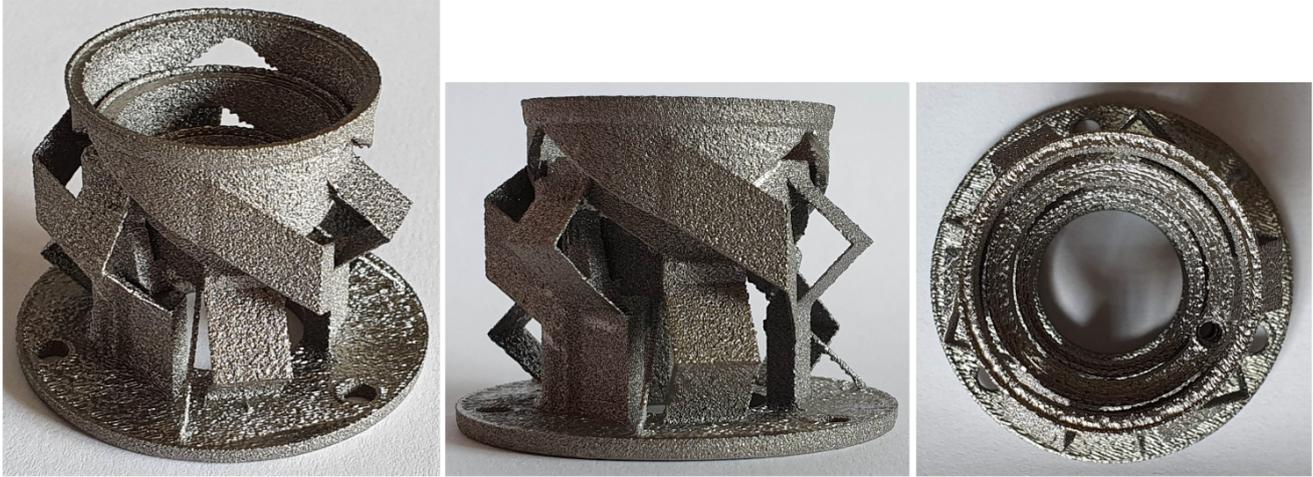
**Figure 30:** Alignment mechanism prototype produced in Ti6Al4V with SLM.
