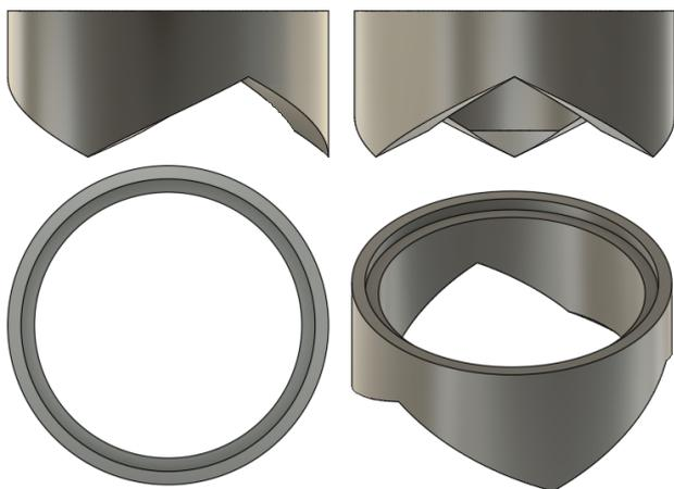
**Figure 22:** Mount for circular optical elements which is self-supporting from three initial points.
