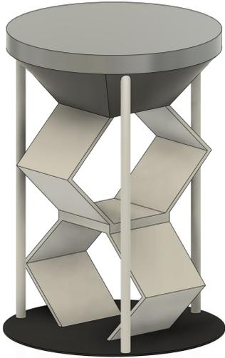
Figure 18: Exactly constrained centering stage building block.
