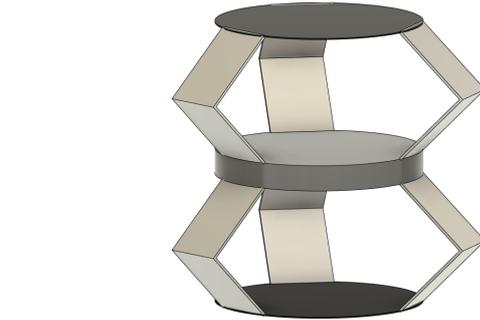
**Figure 16:** Focus stage building block with 6 folded leaf flexures.
