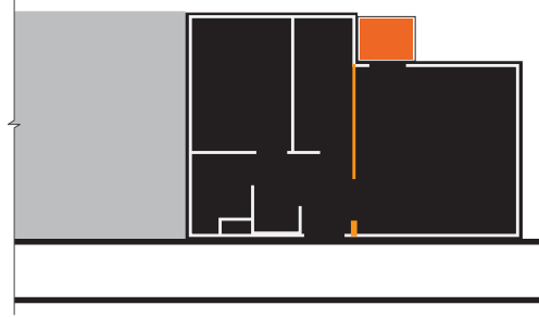
02. ~2020_Agrostone partition demolished and changed to HCB, the wall was also pushed towards the kitchen to get more space in the living room.
