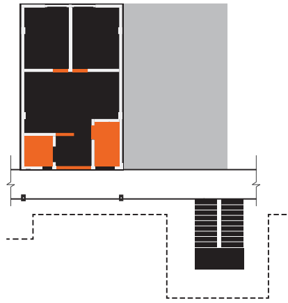
02. ~2012_The family moved in by installing and modifying the doors, removing the HCB dwarf wall, and finishing the kitchen and the toilet
