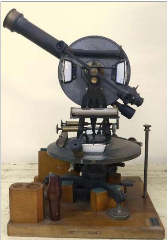
Figure 3: The Hildebrand theodolite used in the early days for the geodetic surveys at Bosscha Observatory and currently displayed in the Exhibition Room at the Observatory (photograph: the authors).
