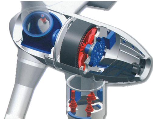
Figure 2.2: Direct drive drivetrain (Jensen et al., 2012)
