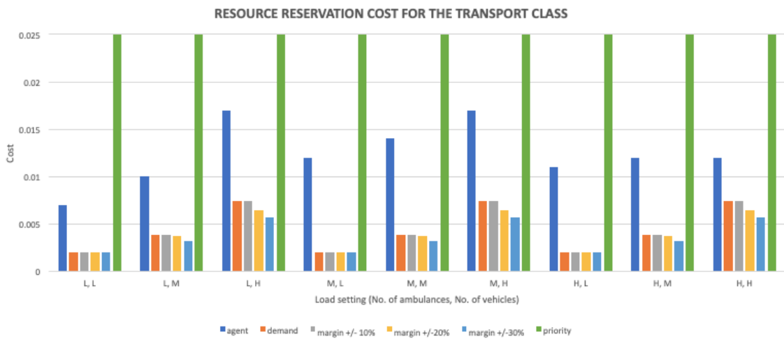
Figure 9.6: Average cost associated with resource allocation in the transport class in Phase 2 for different load settings in the medical and transport classes.
