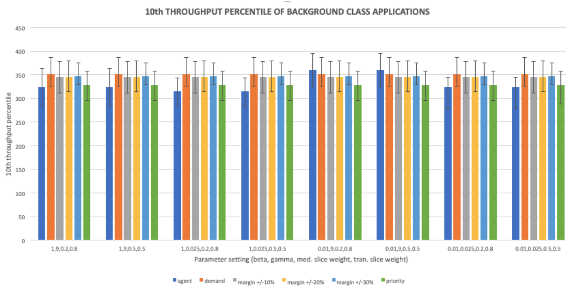
Figure 9.24: 10 th throughput percentile of background class applications in Phase 3 for different settings of evaluation parameters.
