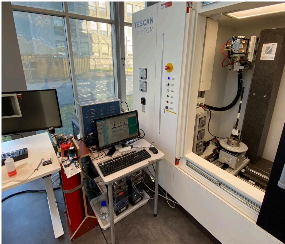
Figure B.5: Experimental set-up outside CoreTOM CT, with the injection pumps visible under the table.
