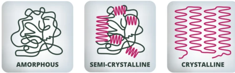
Figure 2.3: A visual representation of the three types of molecular arrangements within a polymer. Reproduced from [5].
