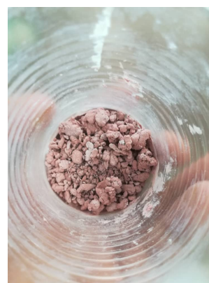
Figure 1: Agglomerated sealant with 5% Al 2 O 3
