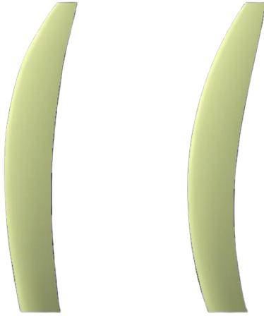
Figure 1.1: Baseline (left) and optimal (right) propeller blade design by Geng et al. - 2021 [8].
