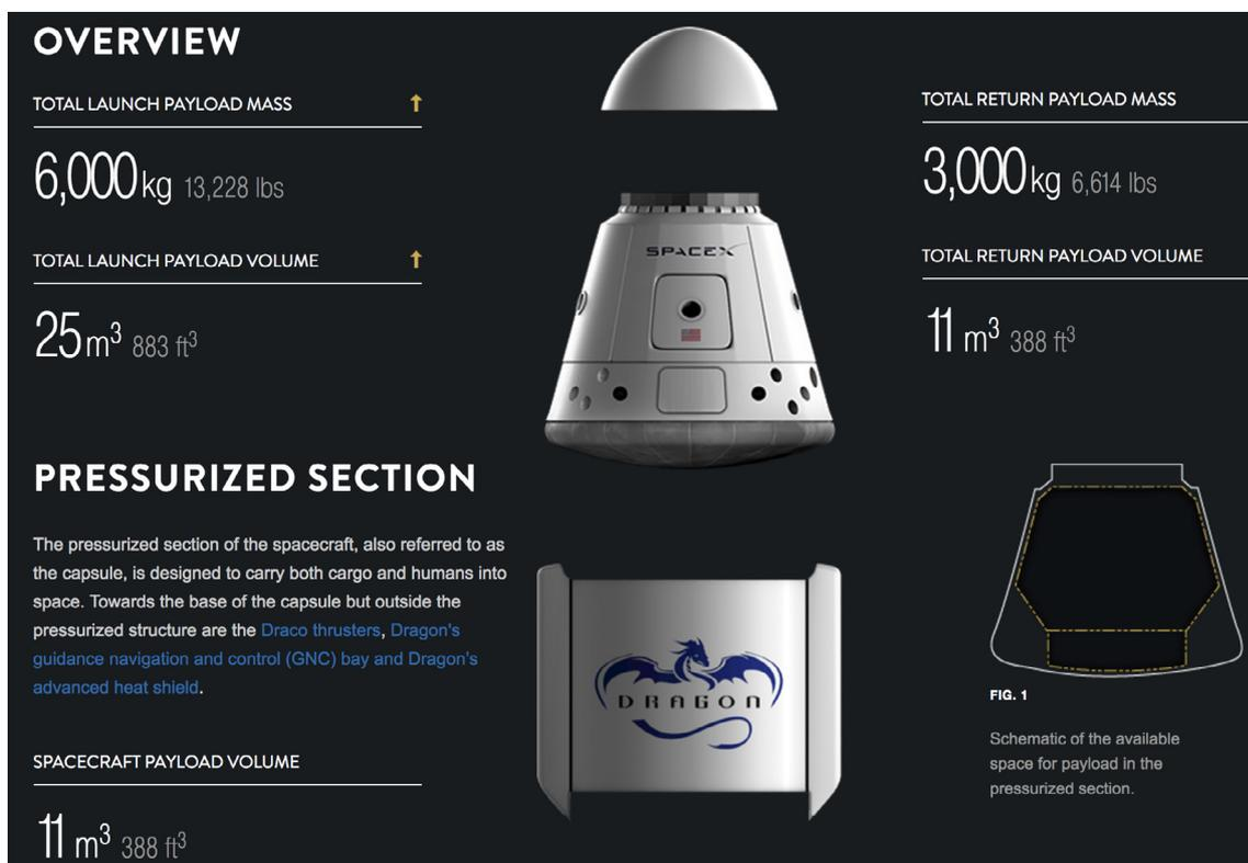
Figure 3.4.7. : Technical Specifications of the Dragon Crew Module (SpaceX, 2017)
