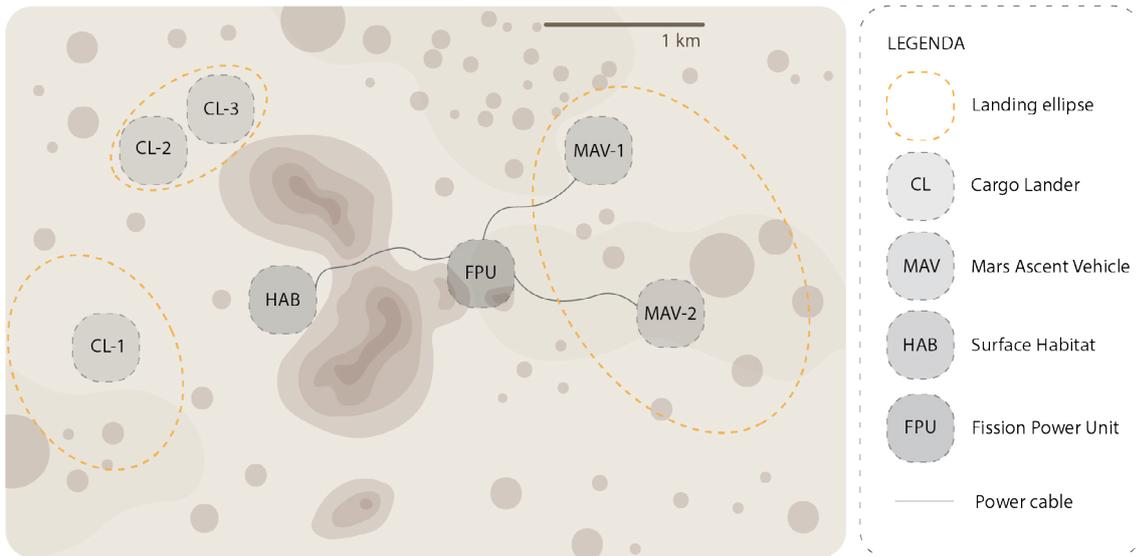
Figure 6.1.1. : Visualisation of chosen site configuration based on DRA 5.0 and the HLS2-workshop.
