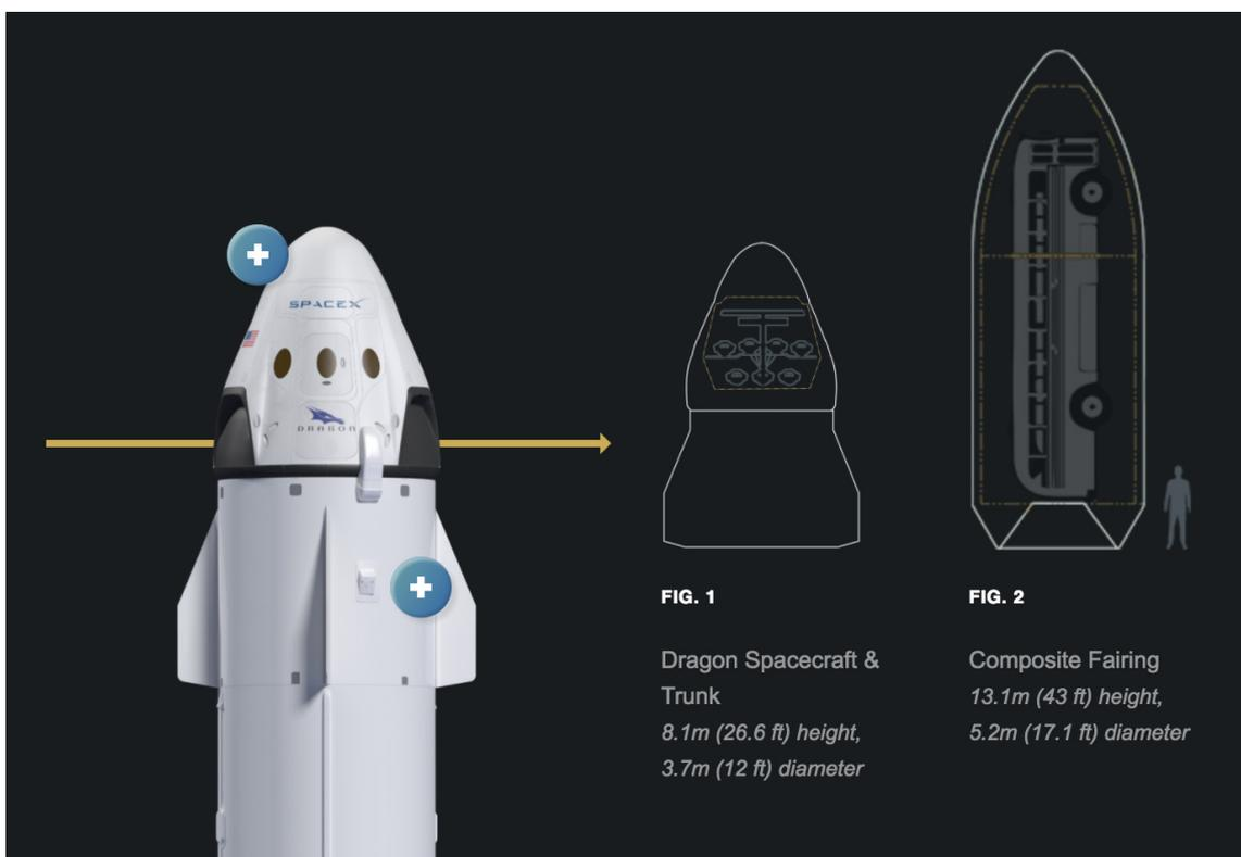
Figure 3.4.8. : Dimensions of modules that can be placed on top of the Falcon (SpaceX, 2017)
