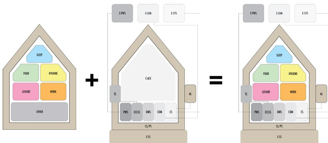
Figure 5.6.3. : The space architect will have to synthesize system configuration and program organization in one integrated design for the habitat.
