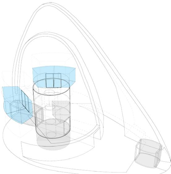
Figure 4.6.8. : The support systems are assumed to create environmental stressors like noise and vibrations. The sleeping quarters are not situated adjacent to the technical spaces.
