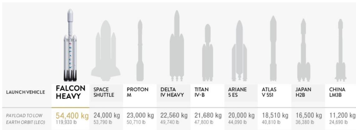
Figure 3.4.6. : Falcon Heavy compared to other space fairing technologies (SpaceX, 2017)
