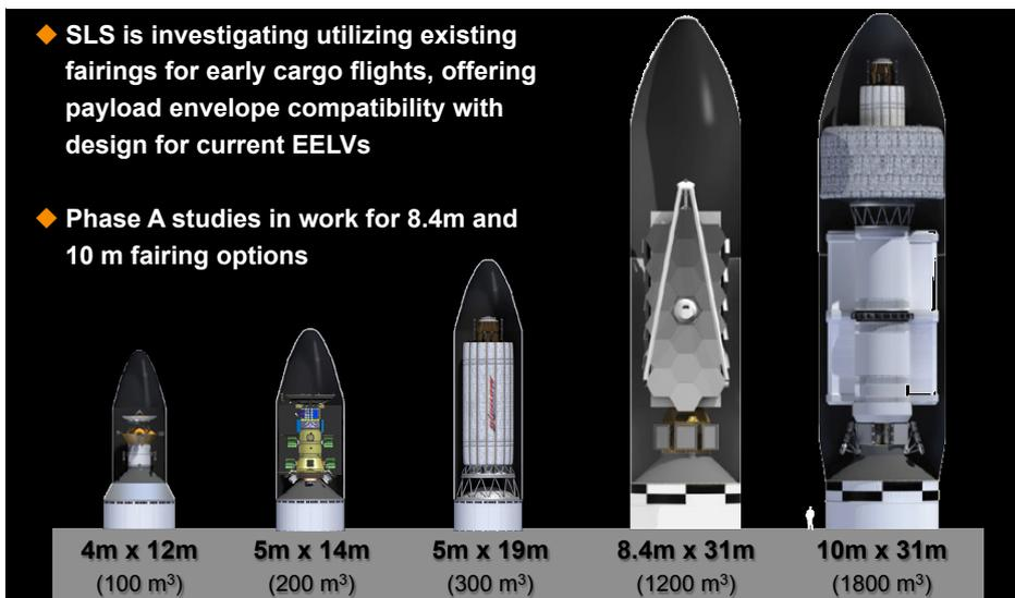
Figure 3.4.4. : Space Launch System capabilities (NASA)
