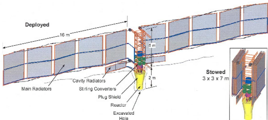
Figure 3.5.10 : Design of a 40 kW Fission Power Unit (FPU) (Rucker et al., 2016)
