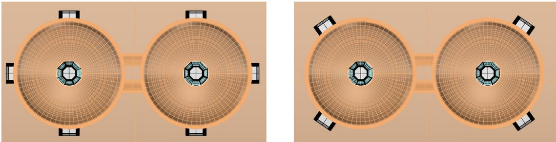
Figure 6.4.2. : A triangular footprint and set-up, as opposed to a cruciform, will result in less molded in airlocks and seems, decreasing the mass and required number of seems of the inflatable membranes.
