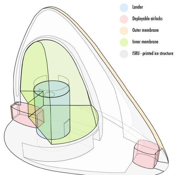
Figure 4.6.7. : Organization of the separate structural elements within the structure.
