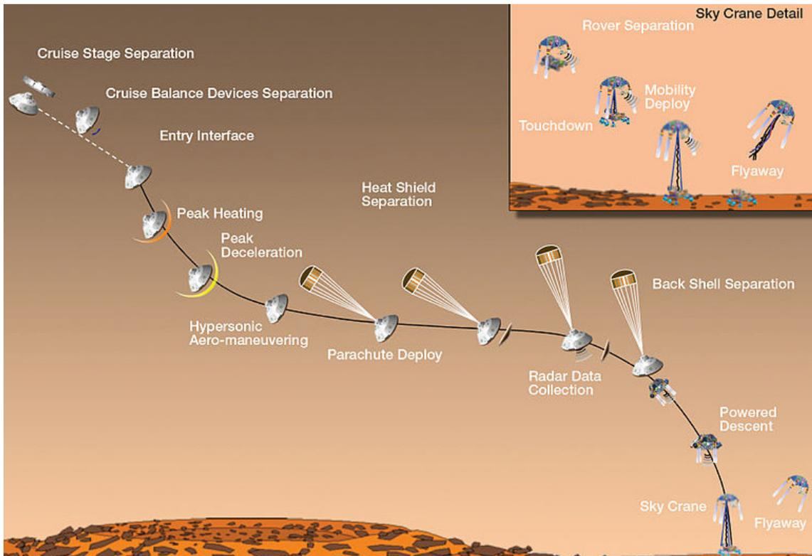
Figure 3.4.10 : Entry Descent and Landing (EDL) sequence of MSL-rover Curiosity (wikipedia, cc)
