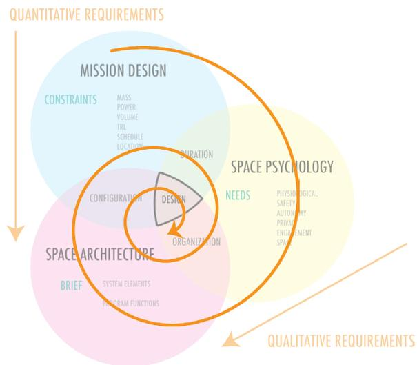
Figure 7.2.2. : Development of the design requires a constant interaction between the various disciplines, meaning that the design process should be organised as an interdisciplinary process between multiple experts with various disciplines and backgrounds.
