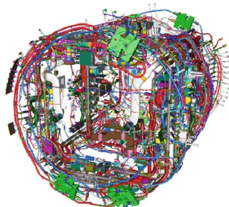
Figure 5.4.2. : Complexity of the ECLSS in Node 2 from the ISS. The complexity of the ECLiSS comes from having to interconnect the ECLSS of six other modules. (Hauptlik-Meusburger et al., 2016)
