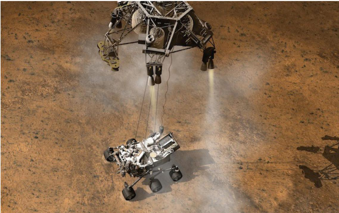
Figure 3.4.12 : Landing of MSL-rover Curiosity with retropropulsion technology (wikipedia, cc)
