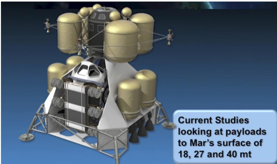
Figure 3.4.19 : Possible configuration of the first cargo lander (NASA EDL, 2017)
