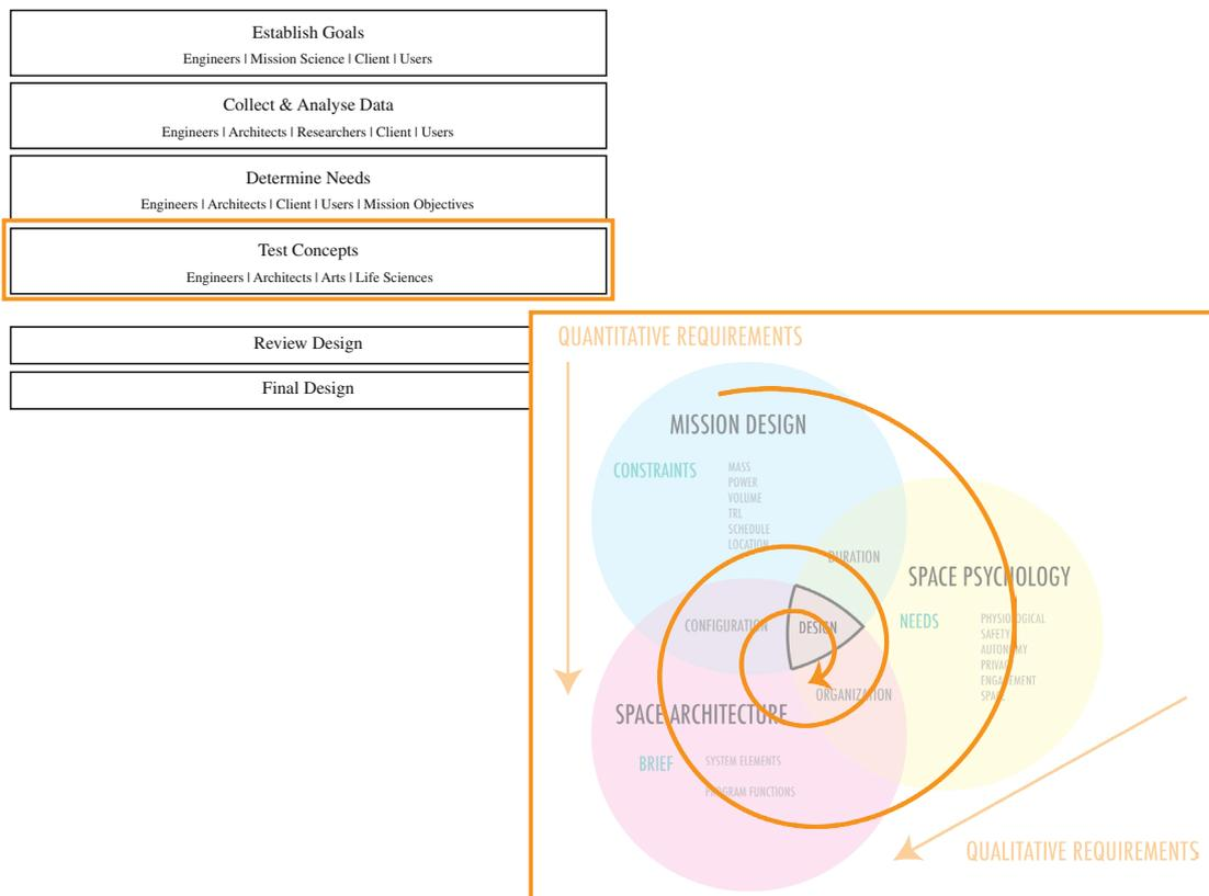
Figure 6.4.5. : During the process of designing and testing of concepts a constant evaluation and iteration should take place between the various involved experts in order to come to a feasible design.
