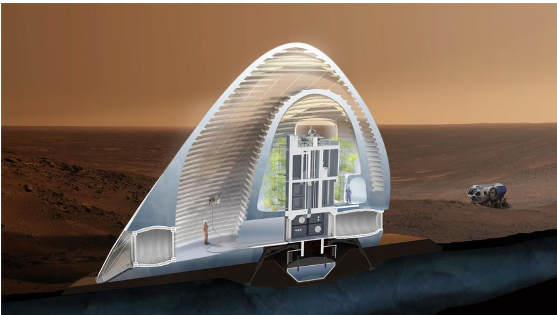
Figure 4.6.4. : Artistic impression showing how the module and inflatable airlocks are placed within the ice structure. Underground, the water is excavated with ISRU technology and stored in tanks.
