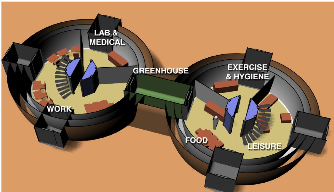
Figure 6.3.1. : Organization of ground floor, work and lab module (left), leisure and exercise module (right)
