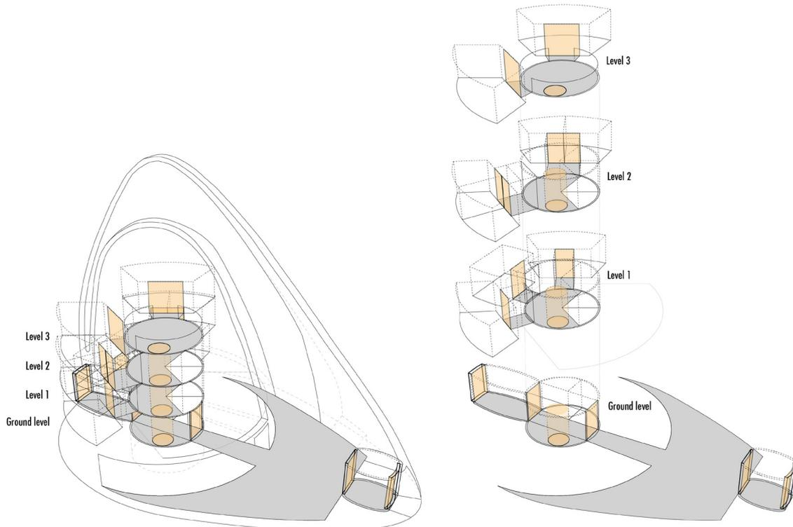
Figure 4.6.10 : Translation paths and doors. All separate program functions can be closed off via doors.
