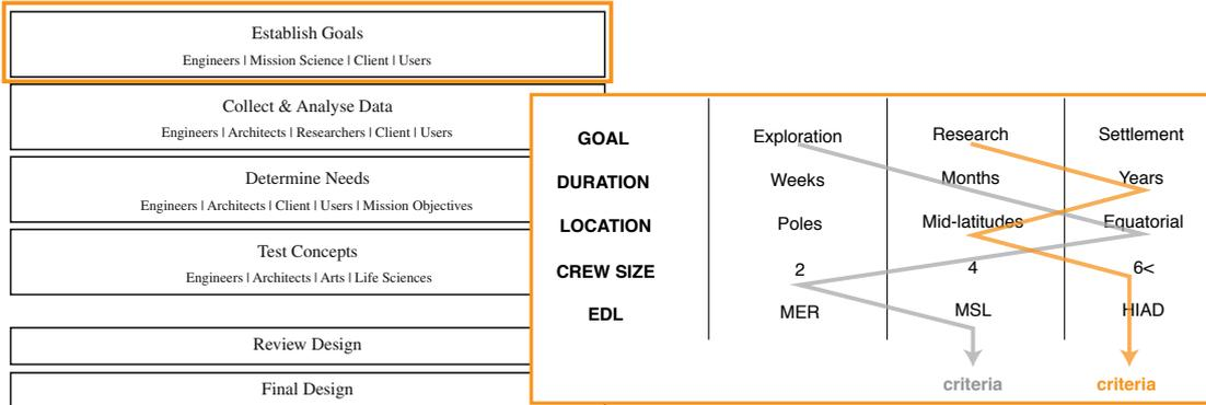
Figure 6.4.4. : Different design decisions in earlier stages related to mission architecture result in other criteria and requirements which in turn change the design parameters for the surface habitat system.
