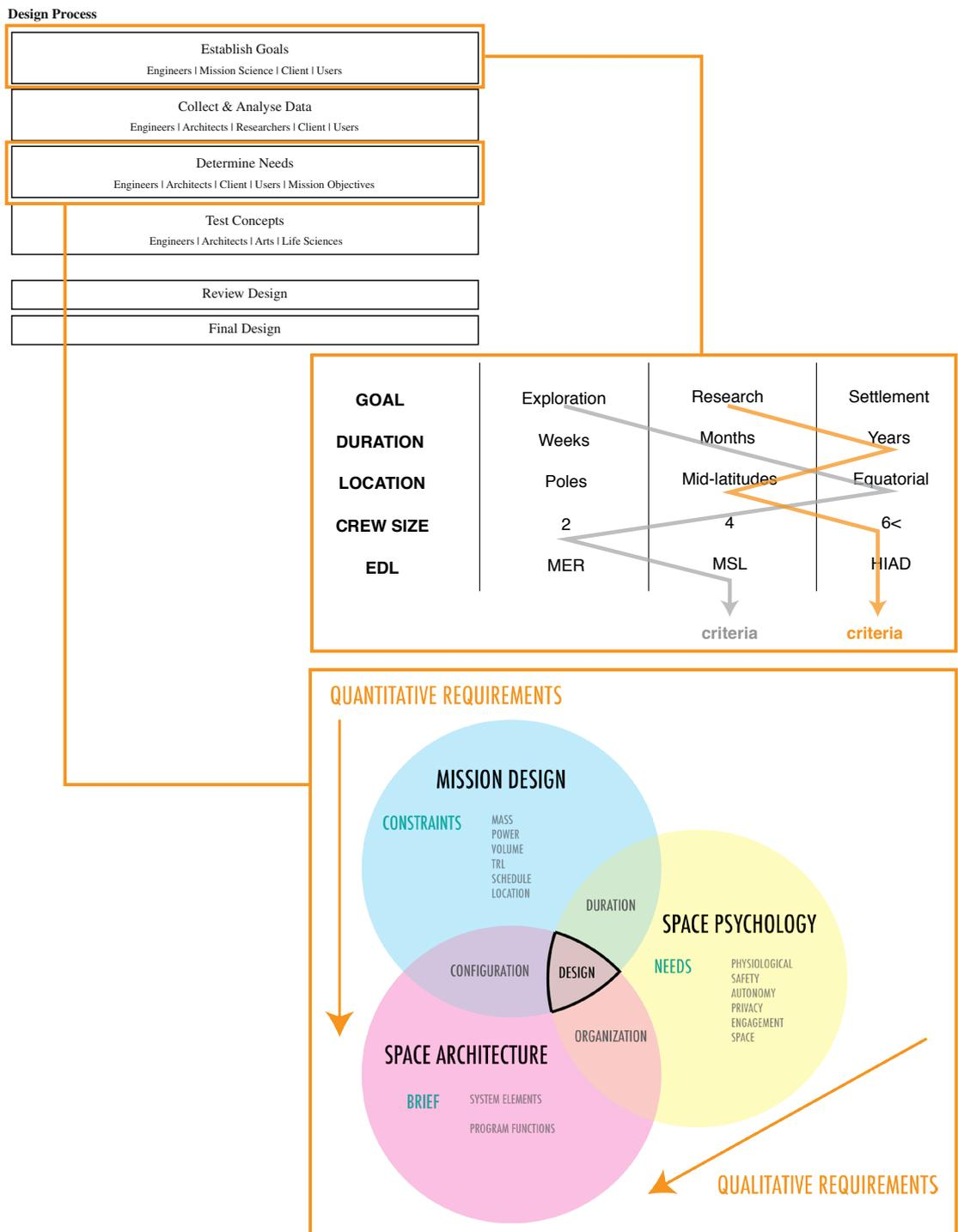
Figure 7.1.1. : Application of the framework in the design process of the space architect with the chosen design parameters based on the research findings.
