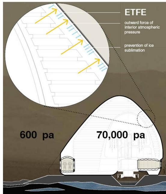
Figure 4.6.3. : Transparent membranes would mitigate pressure differences and ice sublimation.
