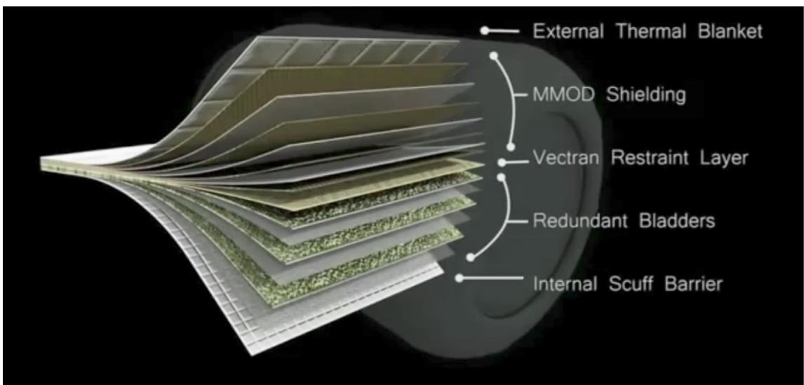
Figure 7.2.3. : The layering of Bigelow's inflatable technology can be used as a starting point and reference for further development of detailing the building construction.
