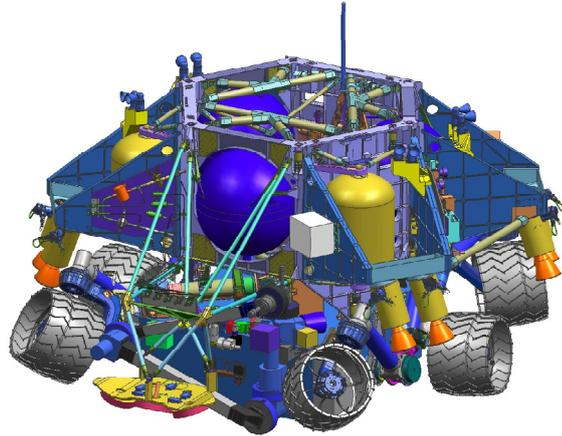
Figure 3.4.18. : Packed configuration of MSL-rover Curiosity (Way et al., 2012)
