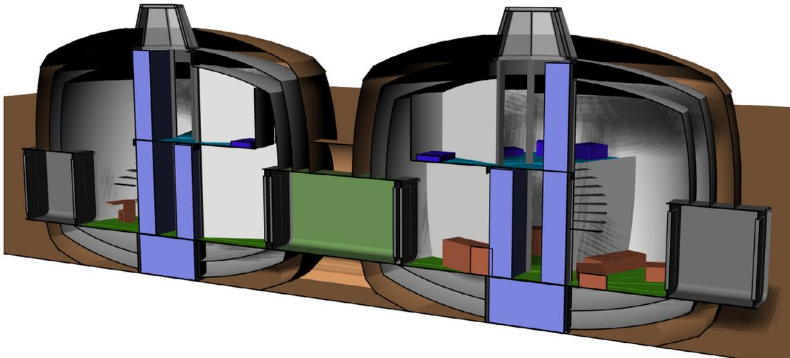
Figure 6.3.6. : Technical space integrated in central module. The green house module forms a transition path between work and leisure activities. Also, the connection module serves a double purpose as a storm shelter.
