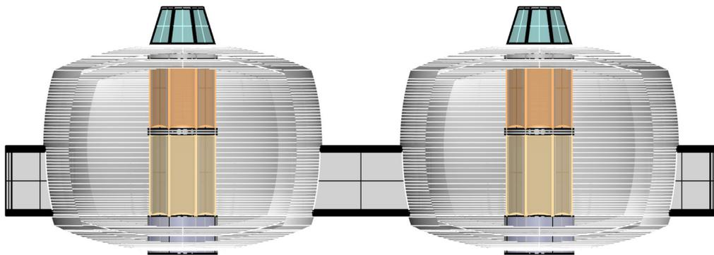
Figure 6.2.2.: Inflate membranes and CO<sub>2</sub>-insulation pockets, connect airlocks to hatches
