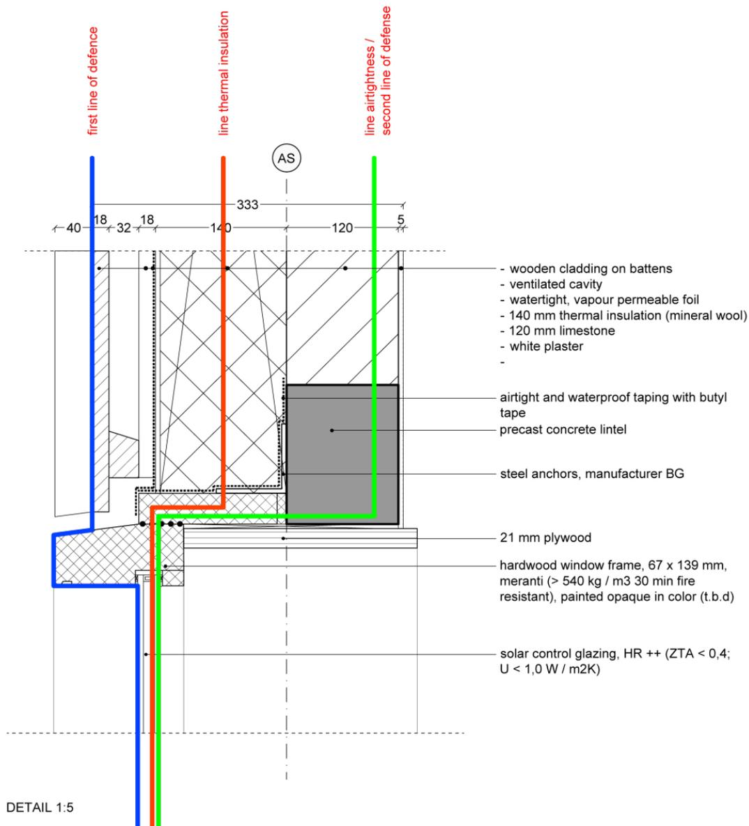
Figure 6.4.1. : A building construction on Earth has to consider the lines and paths for physical requirements of the facade (Bergsma, 2016) A martian facade has to consider similar lines. Yet a major distinction is that in addition, the facade has to consider the lines for radiation shielding, meteoroid impact and an airtight pressurization restraint layer. Also, concerning detailing the joints and seems, abrasive dust has to be considered on Mars.
