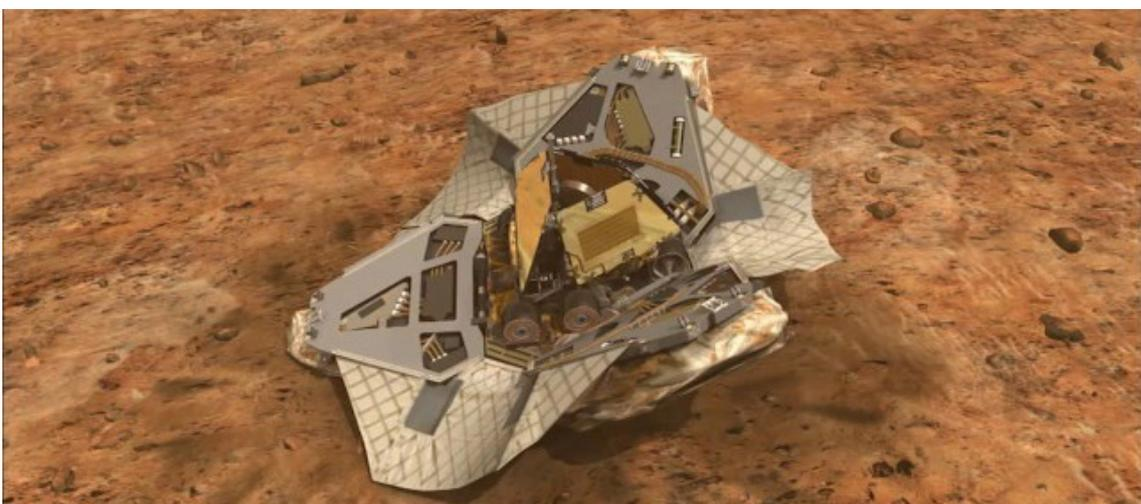
Figure 3.4.15. : Mechanical opening of tetrahedron with deflated airbags. The MER-rover is folded up inside and will deploy its solar arrays and antennas in the next stage of surface operations. (Nat Geo Live, 2015)
