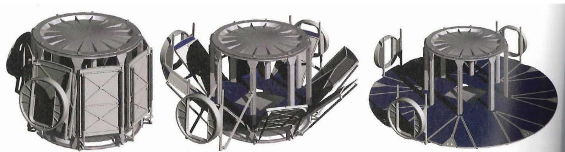
Figure 6.4.3. : The decision of applying integrated foldable floors, drives the floor height and maximum radius of the floors within the module. (A. Scott Howe et al., 2000)
