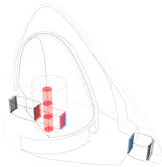
Figure 4.6.6. : Three membranes separate three different pressure zones, each with dual egression, apart from the single staircase leading down in the core of the module.
