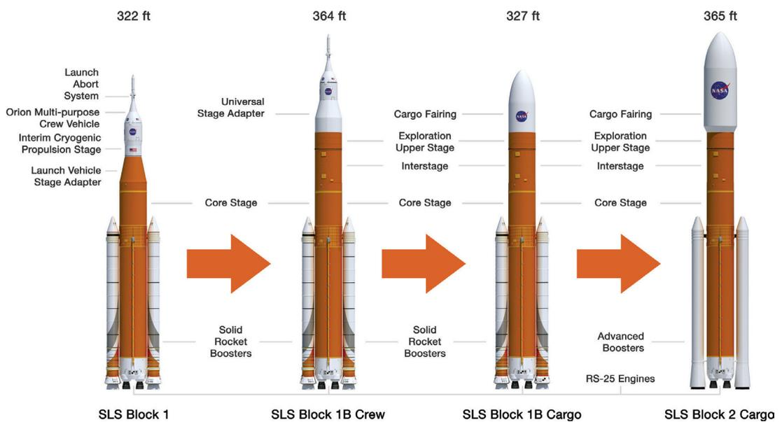
Figure 3.4.5. : Design of the Space Launch System and various scales (NASA)
