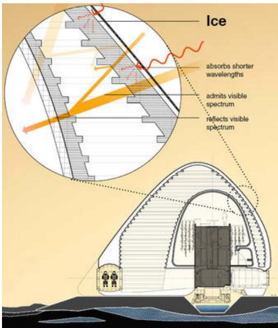
Figure 4.6.2. : The printed ice structure would absorb radiation and admits natural light.
