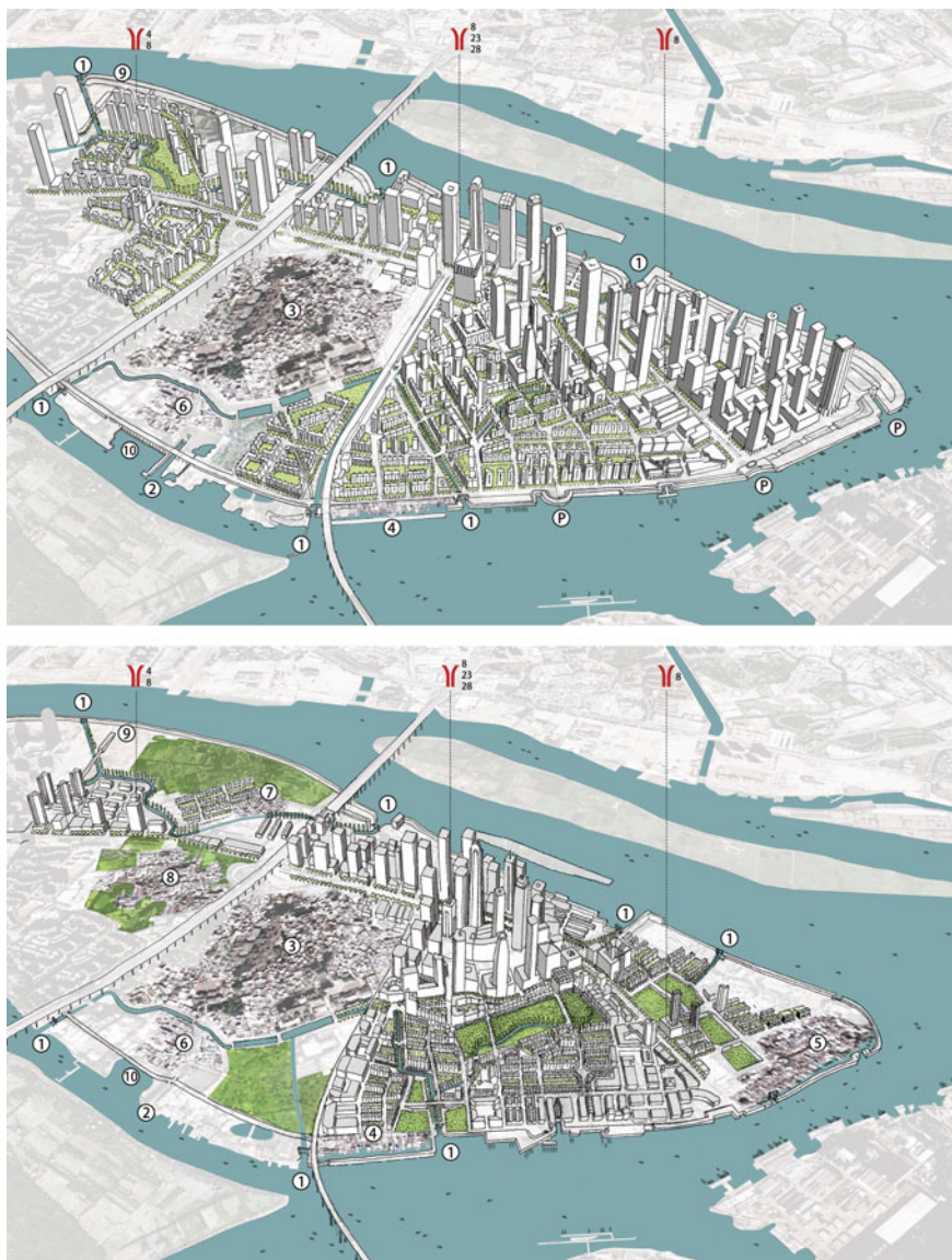
Fig. 7.10 A high development scenario for East Pazou Island (top), and a moderately high development scenario concentrated at three subway stations (below). Existing low-lying land amounting to 80 hectares would remain undeveloped and would be designed to store floodwater after monsoon and tidal surges (Bosselmann et al. 2019)
