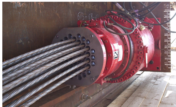
Figure 33: Application of a strand jack (Mammoet).
