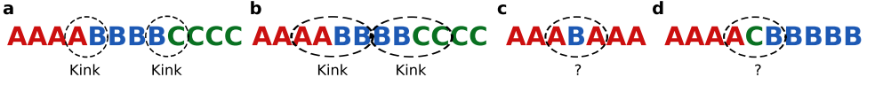
Figure 2.8.: Domain wall characterization in the 3-state Potts model. (a) In the standard definition, a kink is counted whenever two consecutive sites occupy different local states. (b) In the "isolated kink" definition proposed in this work, a kink is only counted when two differing spins are also aligned with their nearest neighbors, ensuring that the adjacent domains have a minimum length of two. (c) A single spin-flip is interpreted as a double kink under the standard definition, but is excluded in the isolated kink definition, as it does not alter the structure of the surrounding domain. (d) A spin-flip occurring at the boundary between two genuine domains is counted as a double kink in the standard approach. In contrast, the isolated kink definition count it as a single kink, since only two true domains are present in the configuration.
