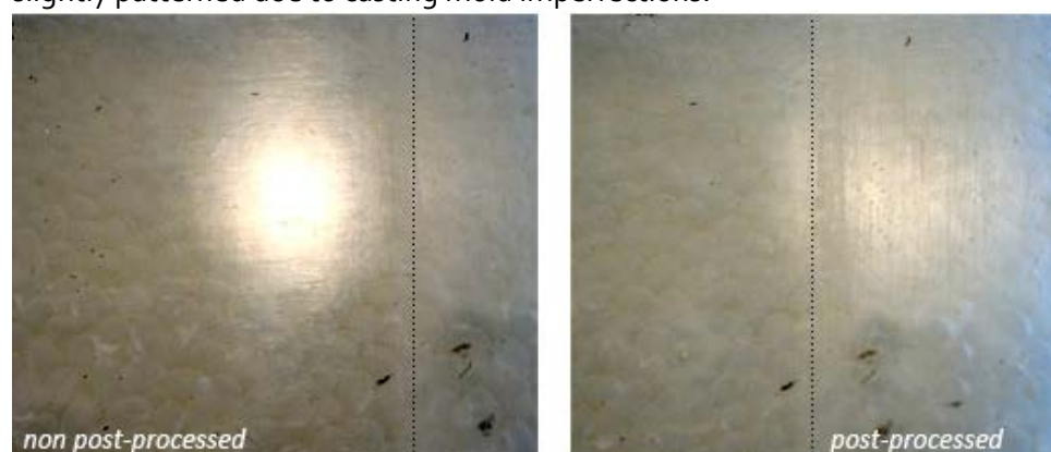
Figure 38: Good surface quality (left) and not good surface quality (right). Sanding the sample to get a more homogenous surface using 3 sand papers in the following sequence: Very Fine: P280, Super Fine: P1000, Ultra-Fine: P2000
