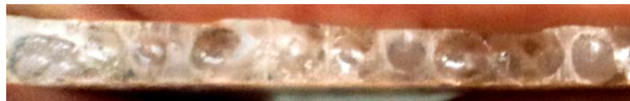
Figure 46: A cutout section of the PEPEP sample, with the PEP capsules removed. Thickness 3.20 mm
