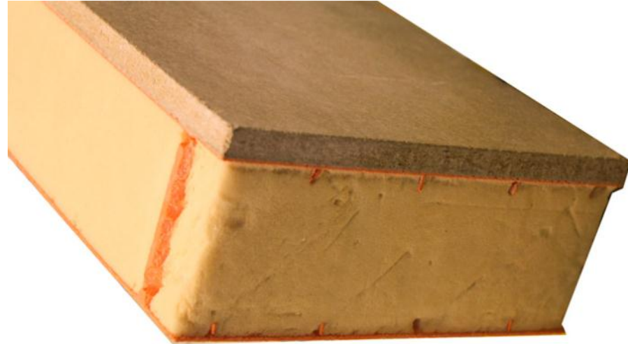
Figure 79: A 75mm GFR polyester panel, with a 20mm cement fiberboard layer attached at its interior surface.
