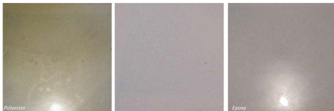
Figure 27: Translucent sheets made of casted Polyester (left) and Epoxy (right) resin, photographed on a grey background (center)
