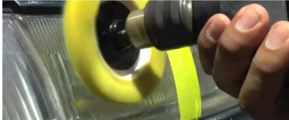
Figure 39: Polishing an acrylic headlight (source: www.youtube.com/user/meguiarsasia?feature=watch )
