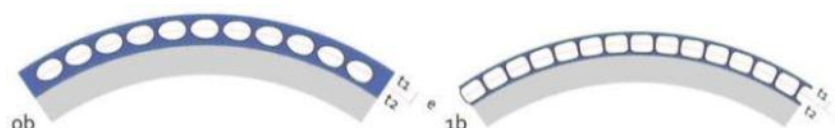
Scheme 28: Optimization using a vacuum, for a slender panel, similar to process described at PEPEP panel
