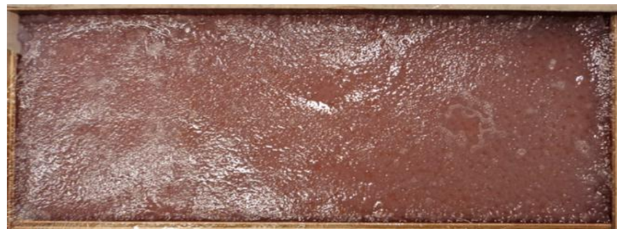
Figure 49: The sample PEPEP2 had two 160\text{gr/m}^2 WR GFR mats at its both sides.
