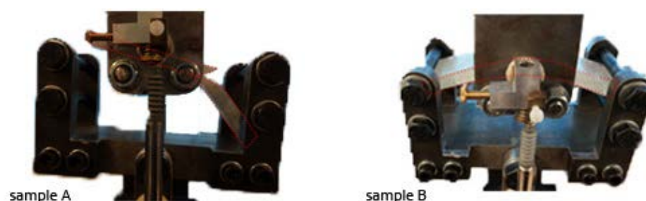
Figure 57: Pictures at the fracture (sample a) and maximum displacement of the 4-point-bending machine (sample b), at left and right respectively.
