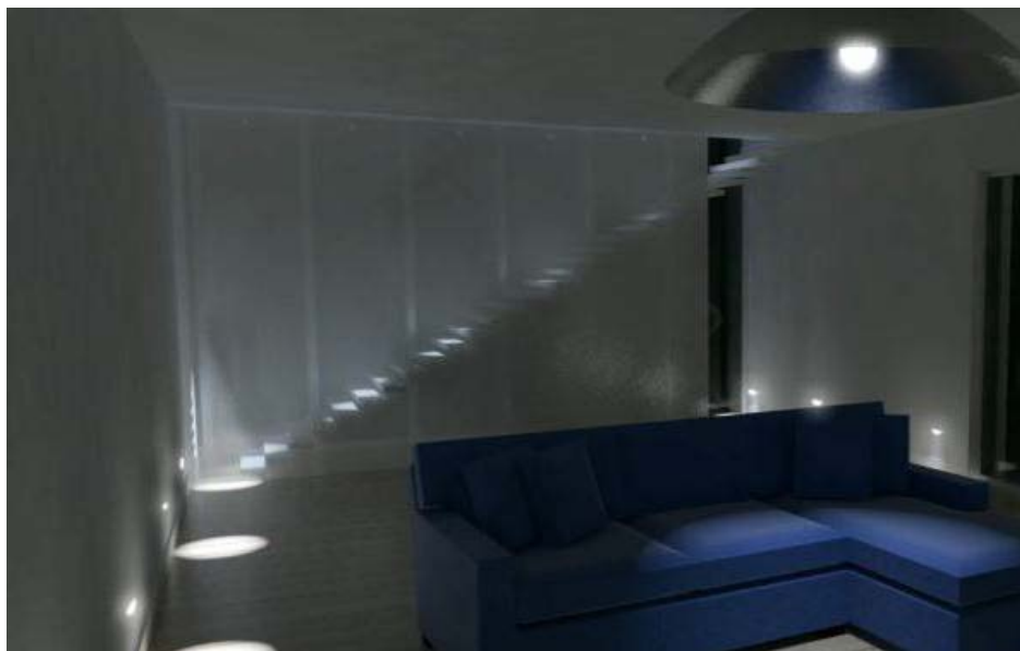
Figure 88 Figure 89: A PEP-GFRP wall can replace a massive slate wall as a heat sink, while at the same time allow for visual connection to the exterior. PCM at its liquid state.
