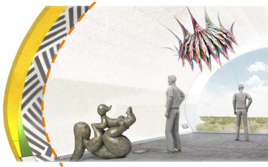
Figure 81: PEPEP panel B with at a museum, integrated at its shell, during morning hours. The pattern selected is a 'fishbone'. Due to higher heat flow at ceiling it will start becoming transparent sooner than the walls.
