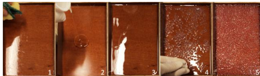
Figure 43: Manufacturing process 1. The PVA release agent is applied to the mold and left to dry for 20 minutes. 2. The mixed EPO+catalyst resin is cast at a first layer. 3. PEP is spread. 4. The final EPO layer is laid, to close any gaps at the surface.
