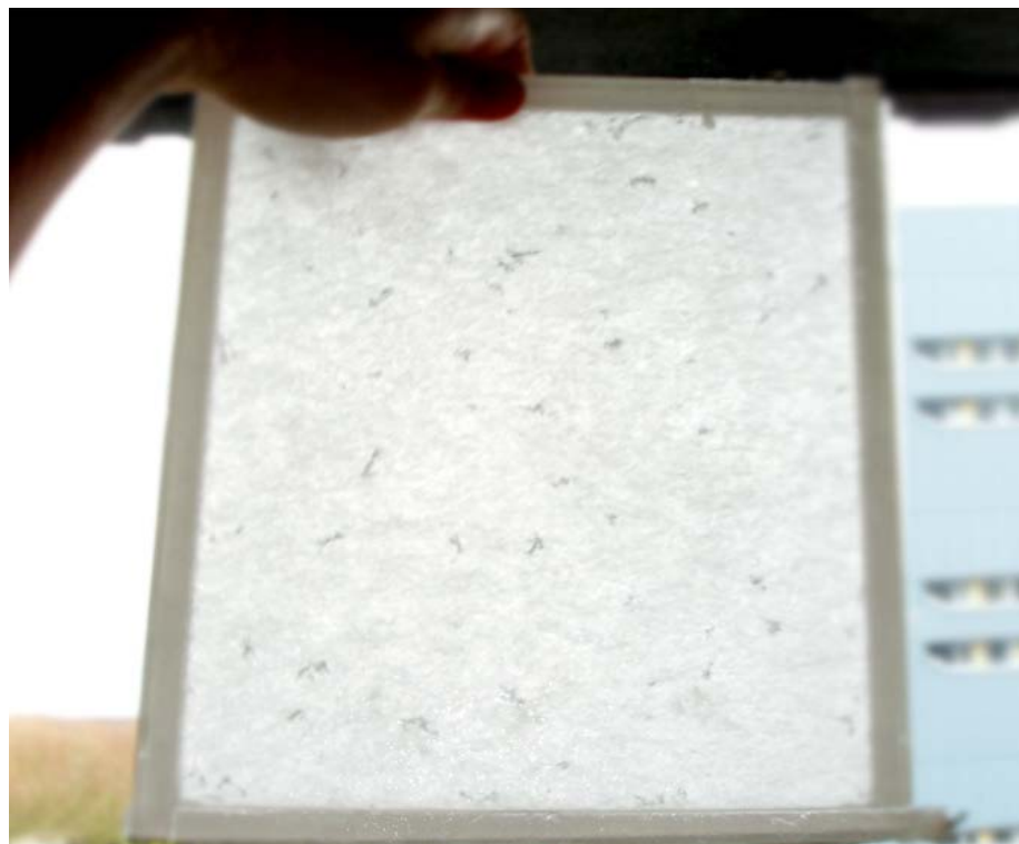
Figure 70: The 12mm PCM-GFRP panel at its Solid state against a window, with a diffuse sky.
