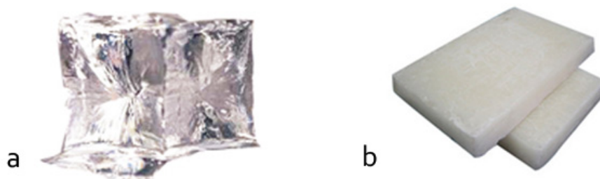
Figure 10: A Hydrated salt (Inorganic PCM) on the left, and a Paraffin Wax (Organic PCM) on the right, both at solid state (source: (left) blogs.indium.com , (right) www.hellotrade.com )
