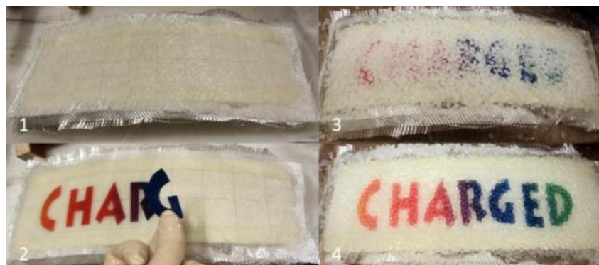
Figure 52: Manufacturing process 1. The Glass Fiber layers were laminated with EPO resin on the bent PET foam, 2. Paper cutouts were inserted before the last fiber layer, 3. The PEP capsules were spread, 4. EPO resin was cast
