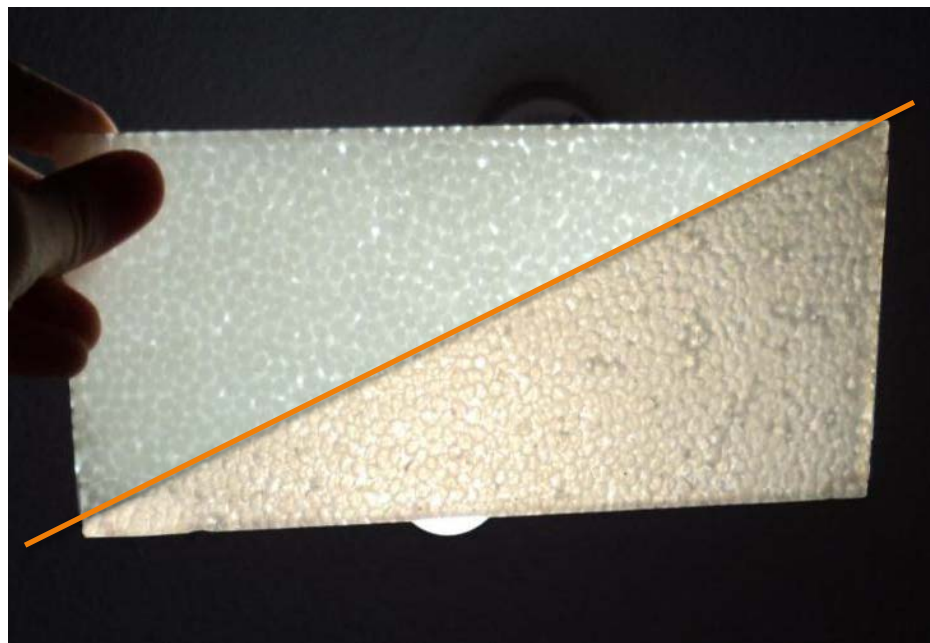
Figure 75: The 8.3mm PEPEP PCMs panel at its Solid and liquid state in front of a 40W incandescent light bulb.
