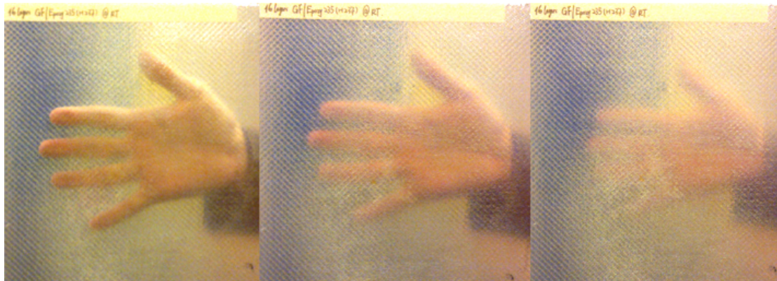
Figure 9: A translucent GFRP laminate using an Epoxy resin as its polymer matrix.
